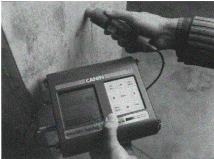
Figure 4.4 (a) A half cell and 'Canin' logging voltmeter. Courtesy of Proceq SA and Hammond Concrete Services.
