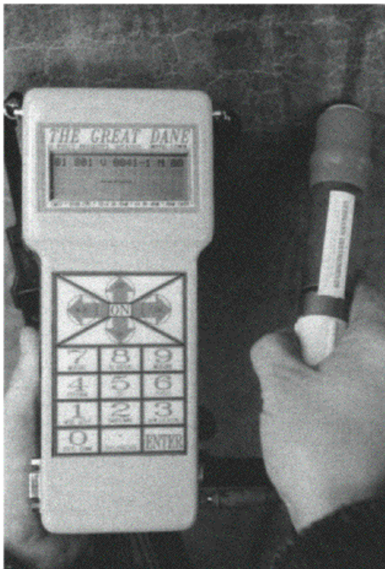
Figure 4.4 (a) A half cell and 'Canin' logging voltmeter. Courtesy of Proceq SA and Hammond Concrete Services.
