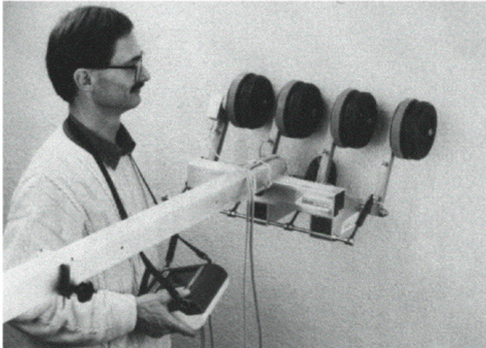
Figure 4.4 (d) The 'Canin 'multiple wheeled half cel array. Courtesy of Proceq SA and Hammond Concrete Services.
