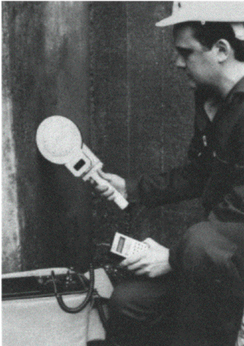
Figure 4.4(c) The potential voltmeter for half cell potential measurements Courtesy CNS Electronics
