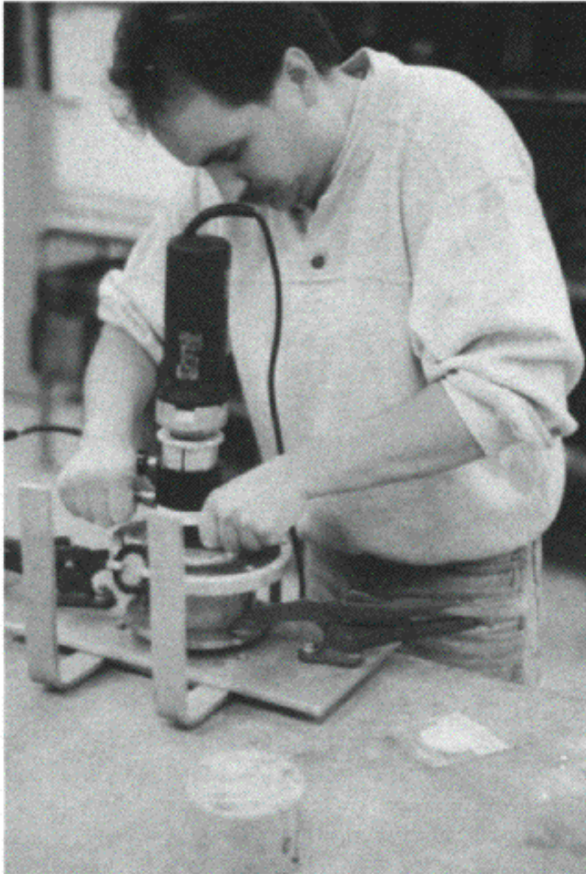
Figure 4.9 The RCT profile grinding kit used in the lab to evaluate the chloride diffusion coefficient of a concrete mix. The grinding may also be done in situ.
