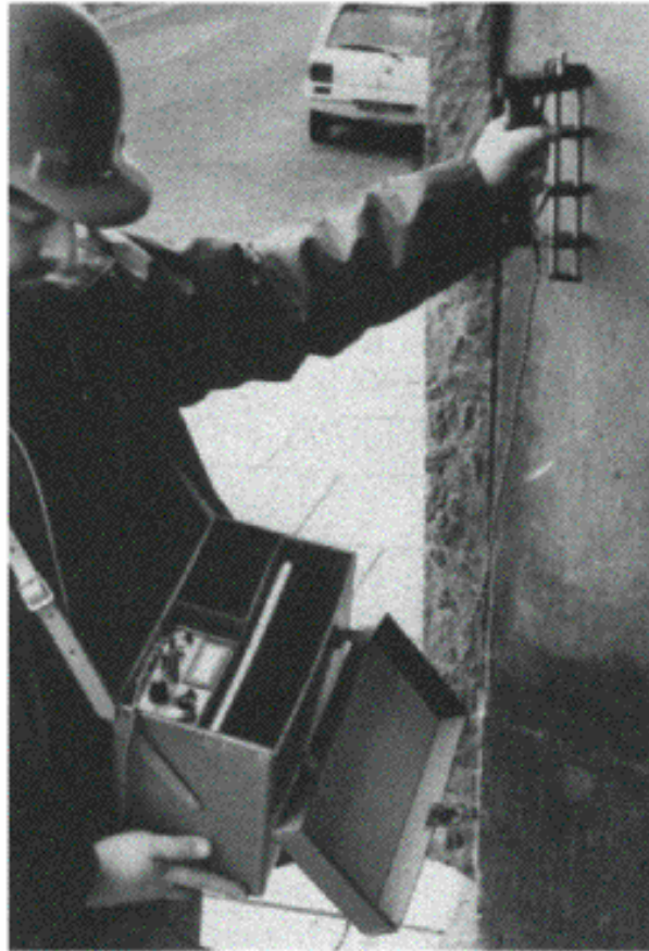
Figure 4.10(a) A four-probe resistivity meter. Courtesy of CNS Electronics.
