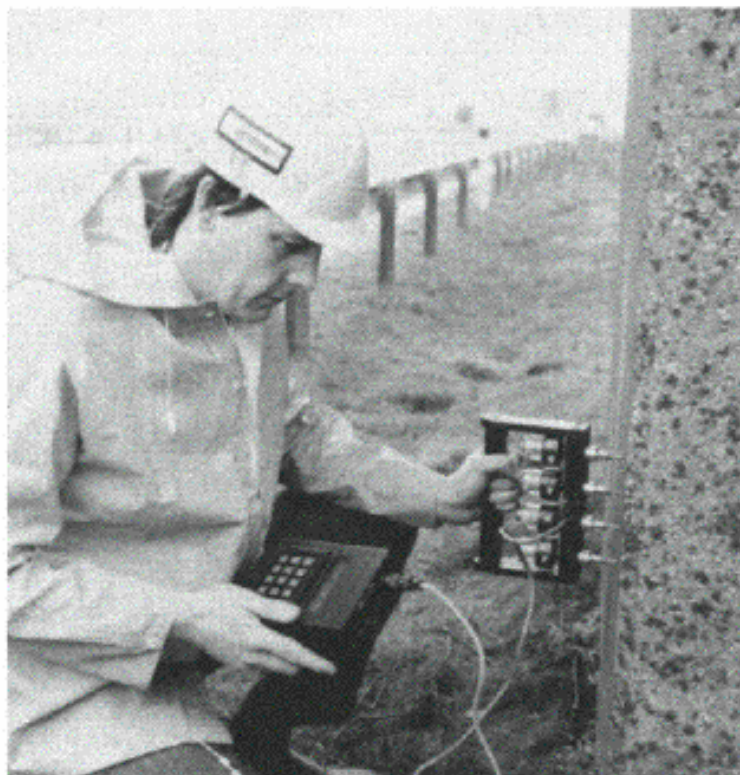
Figure 4.10(b) Four-probe logging resistivity meter with gel contact. Courtesy of Colebrand Ltd.
