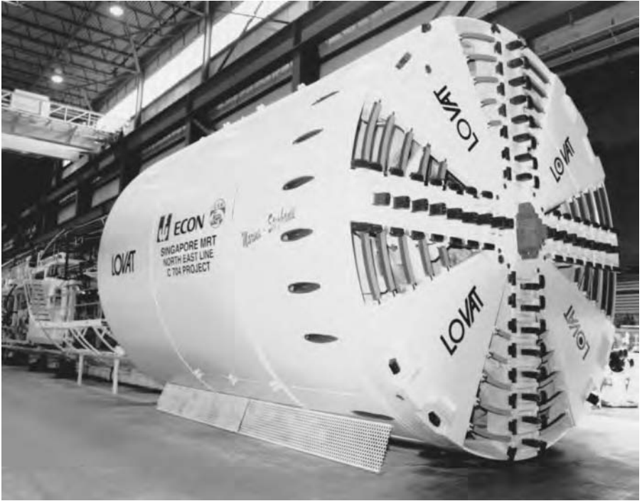
Figure 3.9 Earth Pressure Balance Shield cross-section.
