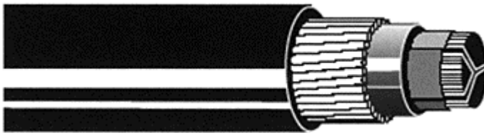
Figure 2.3 Three-phase straight concentric cable
