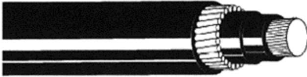
Figure 2.1 Single-core PVC/SWA/PVC cable
