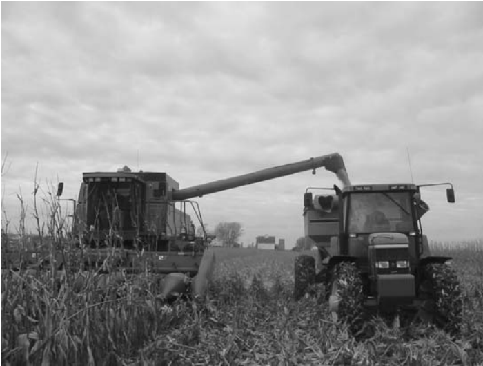
Figure 5.13 Unloading auger extending and moving grain to transport cart.
