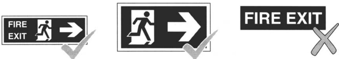
Fig. 1.6 Text only safety signs do not comply.
