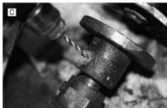
FIGURES 10-18B AND 10-18C. This setscrew is not locked in place. If it comes loose, the propeller shaft will pull out the back of the boat in reverse. It was removed and the shaft was drilled for a through-bolt. Note the flexible coupling in Figure 10-18B , which helps damp engine vibration.
