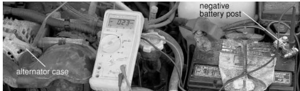
FIGURE 3-29. Testing for voltage drop on the negative side of the charging circuit. It is 0.023 volt—very low.
