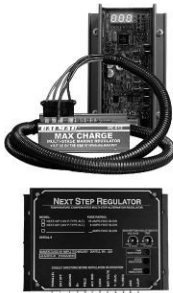
FIGURES 1-29A AND 1-29B. Balmar and Ample Technology multistep voltage regulators. Note the two potentiometer screws on the right-hand side of the Ample Technology regulator. These are for adjusting the absorption voltage and absorption time. Note also the twelve-terminal connector strip at the bottom; wiring these regulators can get quite involved! ( Balmar and Ample Technology )
