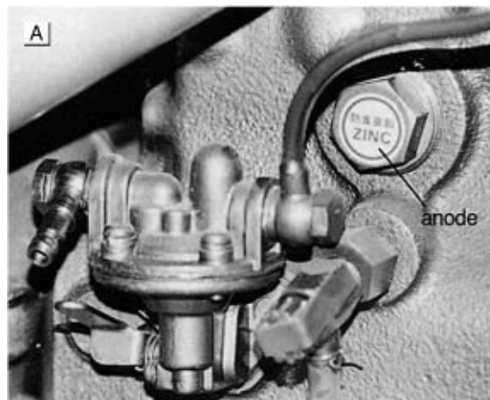
FIGURE 9-14A. A zinc anode in the cooling system of a Yamaha diesel engine.
