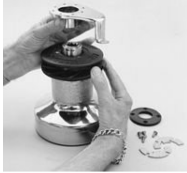
FIGURE 16-16B. Reassembling a self-tailing mechanism. Note the stripper arm being lined up to fit under the feeder arm.
