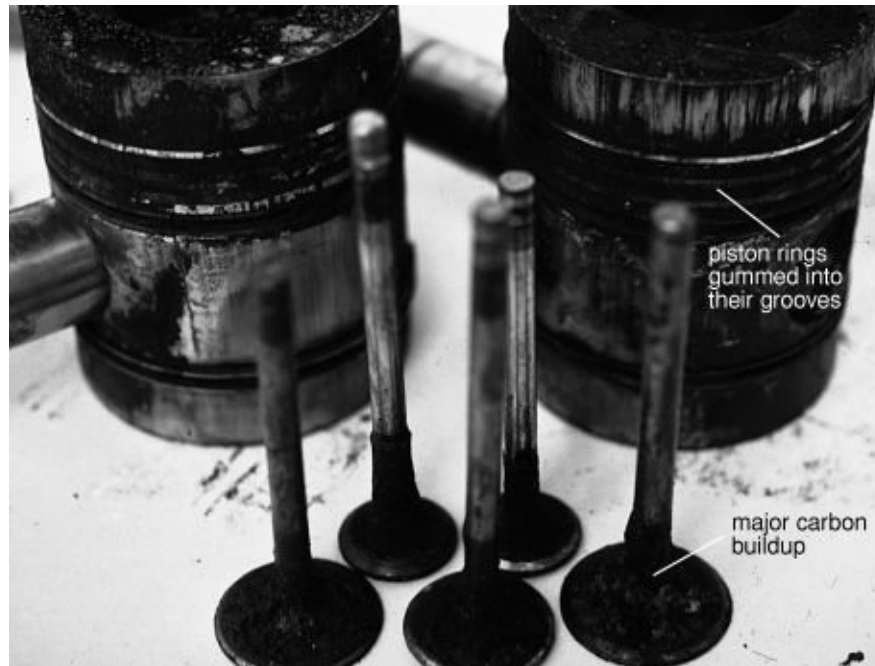
FIGURE 9-4. This engine only has 700 hours on it, but has been completely wrecked by repeated low-load, low-temperature operation.
