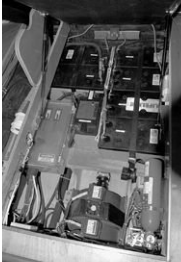
FIGURE 2-20. Diesel/electric installation on a catamaran. The electric motor is in the foreground. This is only half of the battery bank; the other half is in the other hull (which raises certain safety issues).
