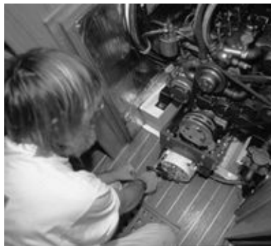
FIGURE 1-25. A 200 amp alternator installed backward on our last boat. To ensure adequate cooling, it is essential to either turn the alternator's fan around or else install a bidirectional fan.
