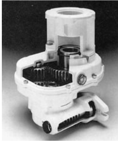
FIGURE 16-28B. The arrangement of the gears in a vertical windlass. ( Maxwell )
