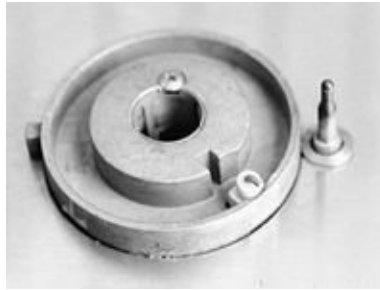
FIGURE 15-8B. The same burner with the burner cap removed to show the spark igniter, which works (and looks) just like a spark plug. The burner nipple is at the bottom of the center hole.
