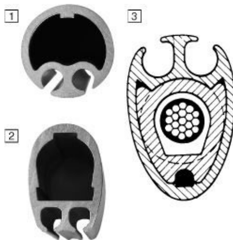
FIGURE 17-53. Roller reefing extrusions. A round extrusion turns
