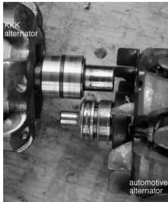
FIGURE 3-22. Automotive alternator versus high-output alternator. Note the difference in the shaft sizes (which translates into different bearing sizes) and slip rings (which translates into electrical load bearing surface). The slip rings on the automotive alternator are badly grooved.
