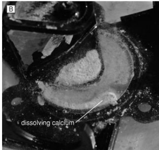
FIGURE 12-32B. Calcium dissolves in undiluted vinegar. Stronger stuff (e.g., muriatic acid) will dissolve it faster.
