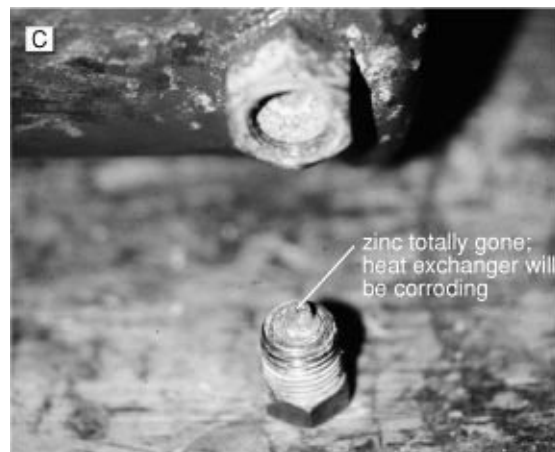
FIGURE 9-14C. This zinc should have been replaced long ago. The heat exchanger is likely corroding.
