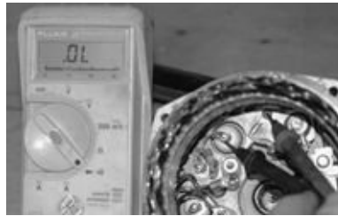
FIGURE 4-9B. The reversal of the meter leads produces an open-circuit reading (“OL”), which is just as it should be (although once again because the diode in question is not disconnected, there is no way of knowing what exactly is being measured).
