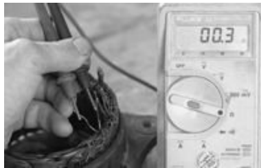
FIGURE 3-41B. Testing between stator coils. There should be a low resistance (in this case, 0.3 ohm).
