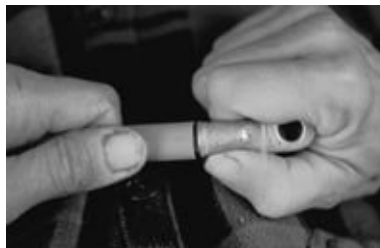
FIGURE 4-59A. Putting a terminal on a large (2/0, 70 mm 2 ) cable.
