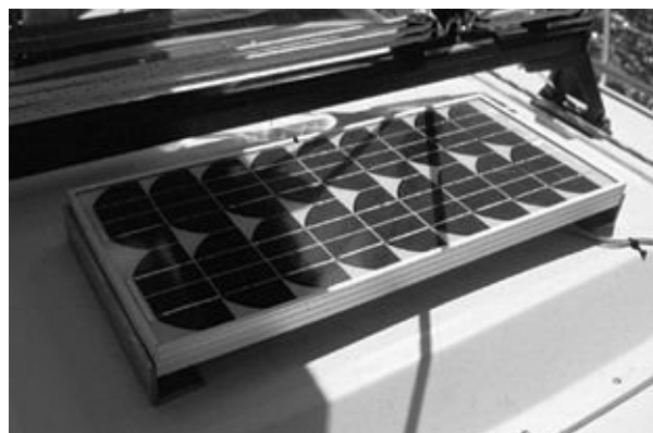
FIGURE 6-45B. Solar panel for keeping the batteries topped off on our old Pacific Seacraft 40. Not an ideal location (because of potential shading) but well protected from physical damage.
