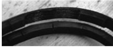
FIGURE 3-26B. Loose belts slip, heat up, harden, and crack.
