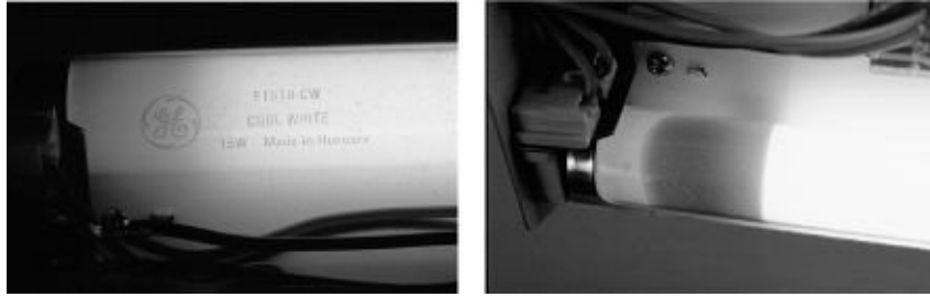
FIGURES 7-32A AND 7-32B. A healthy bulb (no blackening; left) versus one nearing the end of its life (right).
