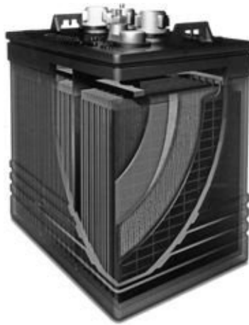
FIGURE 1-2B. Trojan deep-cycle battery construction. Similar to the automotive battery, except that everything is more heavy duty, with considerably more lead, and therefore capacity, in a given volume. (Trojan)
