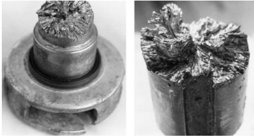
FIGURE 16-19. A windlass shaft sheared by snubbing loads.
