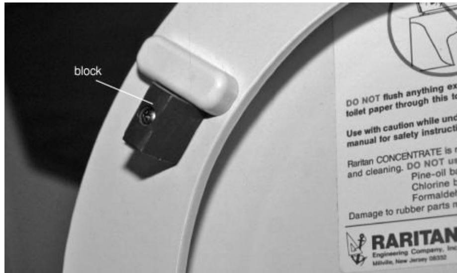
FIGURE 12-30. A block added to the underside of a toilet seat to keep it from sliding sideways and breaking the seat’s hinges.
