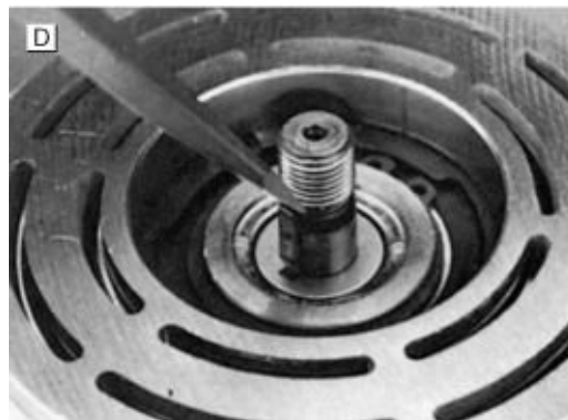
FIGURE 11-39D. 3. Remove shaft key by lightly tapping it loose with a screwdriver and hammer.
