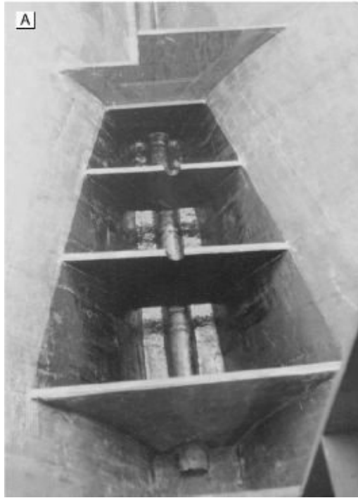
FIGURE 12-2A. Integral freshwater tank construction. The wineglass sections especially lend themselves to integral tanks. The hullside has been lined with a layer of resin-rich mat to seal it (the hull is, in any case, not cored). The half pipe on the centerline is a limber pipe for draining the bilges up forward. Note the spaces below the baffles and the cutout at the top of each to allow for water and air circulation. The baffles (and tank top) are constructed from fiberglass flat stock so they won't be vulnerable to water damage (with an added epoxy-sealed stringer at the top of each baffle to provide a bonding surface for the tank top). The tank has been painted with water tank paint to seal it. This was a mistake (see the text). The area in front of the forward baffle is the boat's sump; forward of this is a diesel tank. Placing the sump between the two maintains total separation of the drinking water tank from the diesel tank.
