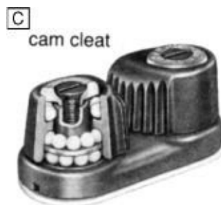
FIGURE 16-2C. Use of bearings in a cam cleat and in the pedestal of a swivel block. ( Harken )
