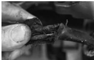
FIGURE 10-13B. A corroded engine control jacket. The inner cable is stainless steel and is just fine, but the spiral-wound outer case is steel that has rusted right through.
