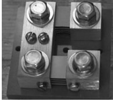
FIGURE 1-39B. A shunt for measuring high amperages.
