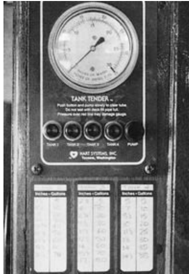
FIGURE 9-50. A pneumatic tank-level gauge. The gauge has been calibrated to the various tanks in the boat, with the relationship between the gauge reading and the tank volumes codified in the tables beneath the meter.
