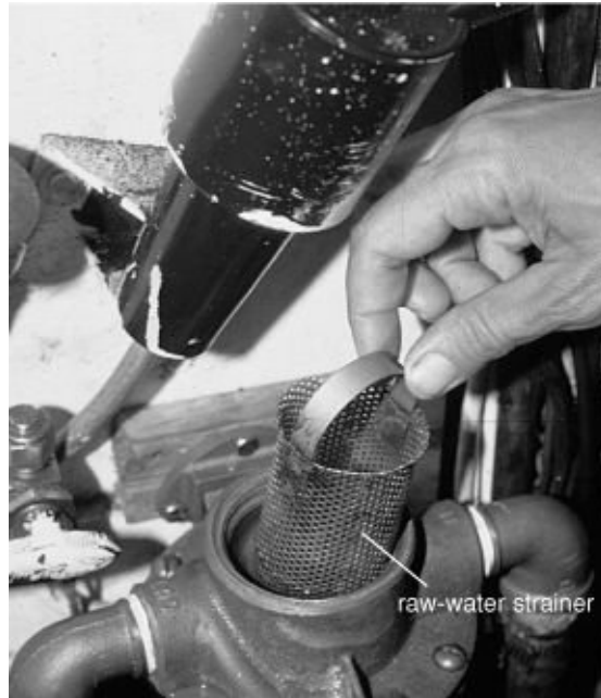
FIGURE 9-36B. Removing the raw-water strainer for cleaning.
