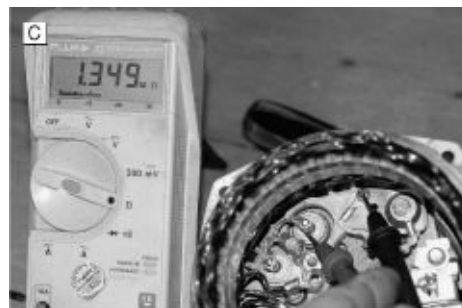
FIGURE 4-9B. The reversal of the meter leads produces an open-circuit reading (“OL”), which is just as it should be (although once again because the diode in question is not disconnected, there is no way of knowing what exactly is being measured).
