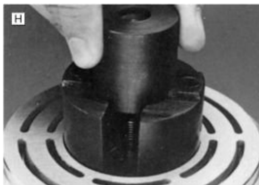
FIGURE 11-39H. 6. Remove rotor pulley assembly. First insert the lip of the jaws into the snap ring groove (snap ring removed in step 4). Then place rotor puller shaft protector (puller set) over the exposed shaft.
