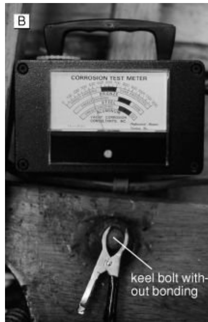
FIGURE 5-18B. A millivolt reading from a keel bolt wired to a lightning grounding system but not connected to a zinc. Note that the reading of -300 mV is close to that given for lead in Table 5-1 .
