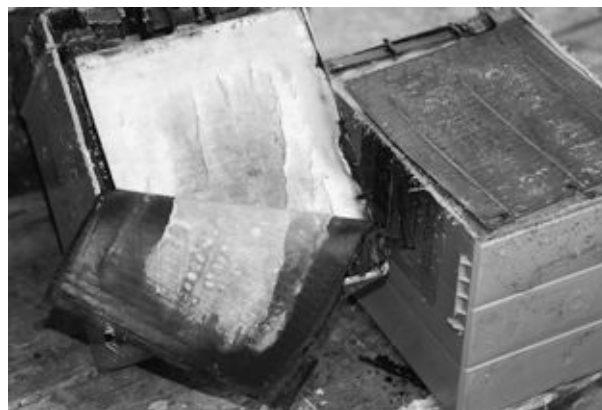
FIGURE 1-6. An AGM battery. Fiberglass mats between the battery plates hold the electrolyte by capillary action.
