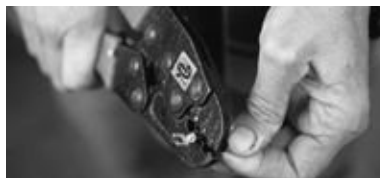
FIGURE 4-57. A ratcheting crimper is an excellent tool that makes it difficult to mess up!
