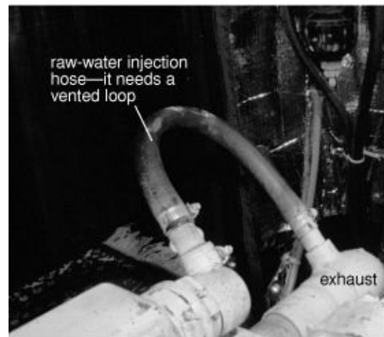
FIGURE 9-16B. Another installation without a vented loop.
