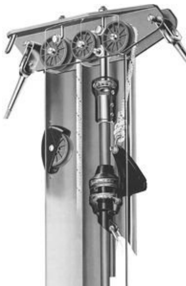
FIGURE 17-64B. A typical contemporary in-mast reefing arrangement. ( Jim Sollers )
