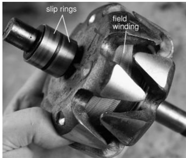
FIGURE 3-18. An alternator rotor constructed to produce multiple north and south magnetic poles.
