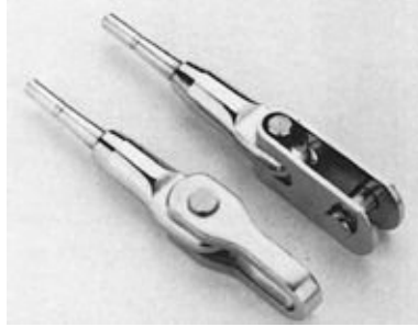
FIGURE 17-30. Fatigue-indicating rod rigging terminals. If the fitting is subjected to undue stress, the upper portion of the sleeve (above the groove) will break away to give early warning of a possible failure. ( Navtec )
