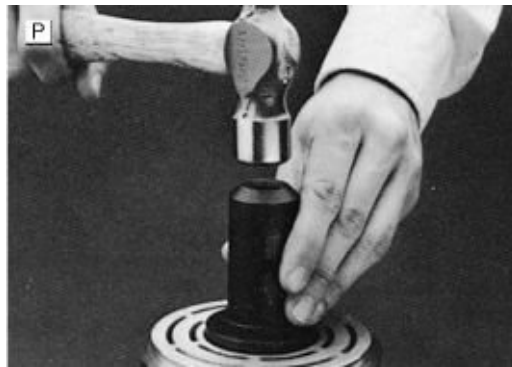
FIGURE 11-39P. Tap the end of the driver with a hammer while guiding the rotor to prevent binding. Tap until the rotor bottoms against the compressor's front housing hub (there will be a distinct change of sound during the tapping process). (3) Reinstall the internal bearing snap ring with pinch-type pliers. (4) Reinstall the external front housing snap ring with spread-type pliers. (5) Replace the front-plate assembly. Check that the original clutch shims are in place on the compressor shaft. Next replace the compressor shaft key, then
