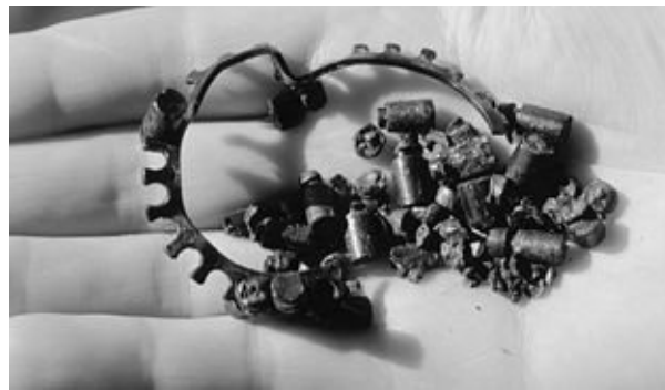
FIGURE 16-4F. A disintegrated turning block. The plastic bearings were not up to the task! This particular block was subsequently redesigned with higher-strength plastic (Torlon) bearings.
