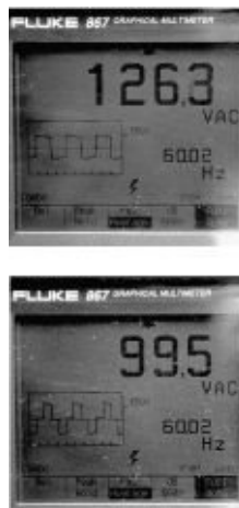
FIGURES 6-18C AND 6-18D. A modified-sine-wave inverter subjected to varying loads at varying battery voltages. Note the wide variation in output voltage (from 126.3 to 99.5) as measured by an averaging meter (as opposed to an RMS meter—see the text), and the changing waveform, but the stable frequency (60.02 Hz).
