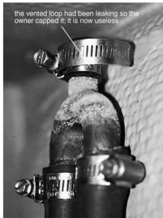
FIGURE 9-16G. This boat has a vented loop that was spraying water into the engine room, so the owner capped the loop and rendered it inoperative!
