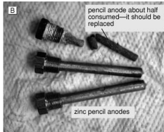
FIGURE 9-14B. Many heat exchangers have zinc pencil anodes. These should be replaced when they are no more than half consumed.
