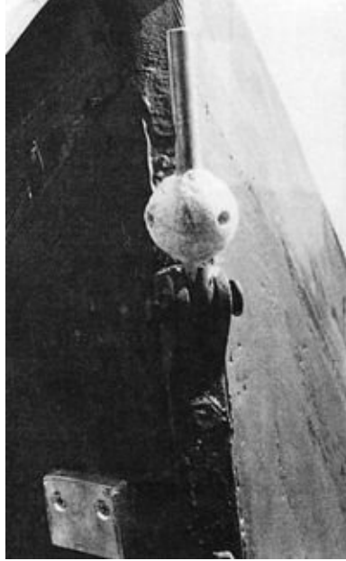
FIGURE 5-19. Destruction of wood due to overprotection of underwater metal fittings. Because of alkali attack, the entire bow area of this wooden boat has had to be heavily patched with epoxy filler.
