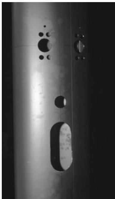
FIGURE 17-17B. A mast under construction. Notice the rounded stress-relieving corners on the cutouts.
