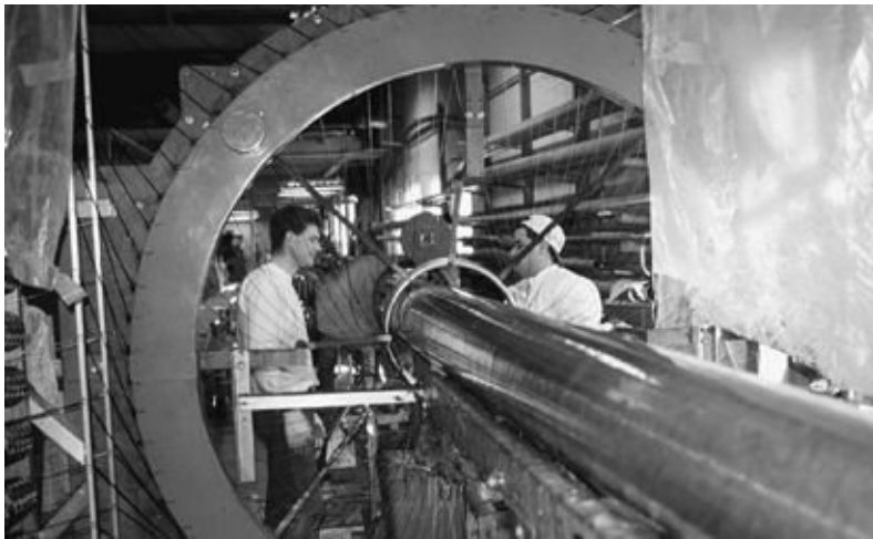
FIGURES 17-22A AND 17-22B. Carbon spars are substantially handmade. The top photo shows a hand layup using prepreg fibers, a very labor intensive and lightweight approach; the bottom photo shows a spar being woven, a less labor intensive and not as lightweight approach.
