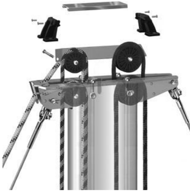
FIGURE 17-18A. A removable head box makes sheave maintenance much easier than on many older masts. ( Selden )
