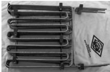
FIGURE 11-14A. The evaporator coil from a Glacier Bay holding plate, with six coils in parallel.
