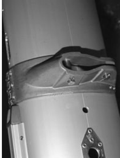
FIGURE 17-16A. This excellent type of spreader socket distributes the spreader's loads over a substantial area of the mast.
