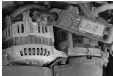
FIGURE 3-31. A clamp-type DC ammeter—a very useful tool—on a nominal 60 amp alternator.
