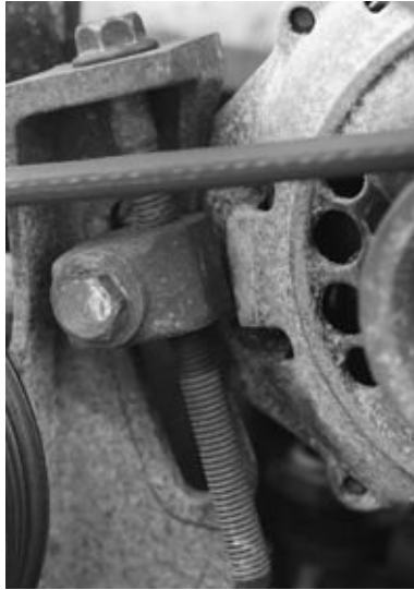
FIGURE 3-25. A belt-tensioning device built into an alternator bracket.
