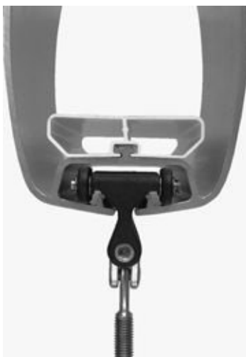
FIGURE 17-19. Selden's in-mast car for a fully battened mainsail. ( Selden )
