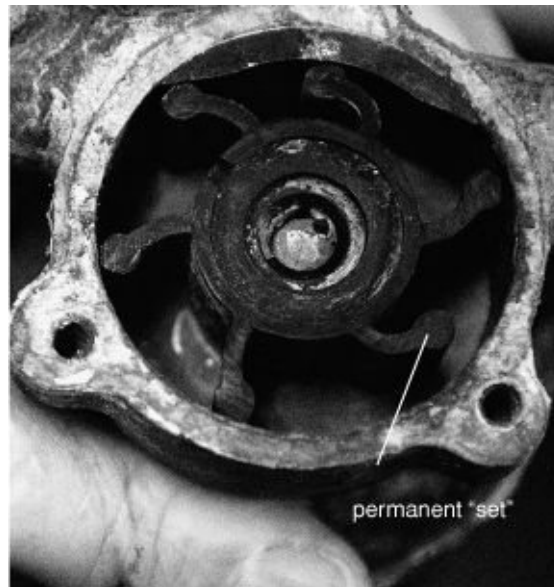
FIGURE 9-37H. Even though the impeller tips are still curved, if the vanes retain a “set” after removal, the impeller needs replacing.
