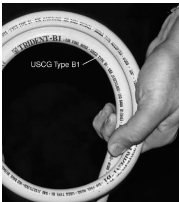
FIGURE 12-19A. A properly labeled fuel hose.
