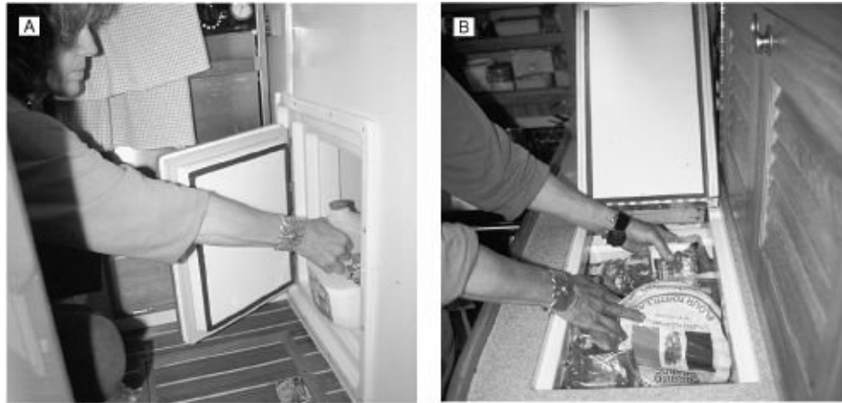
FIGURES 11-8A AND 11-8B. The convenience of a front-opening icebox (11-8A) versus digging through the contents to find something (11-8B).
