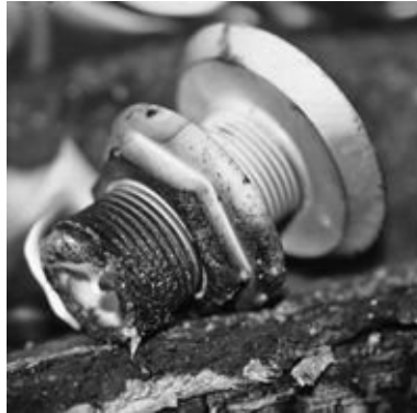
FIGURE 12-44. Even fire-retardant plastic through-hulls will burn if enough heat is applied.
