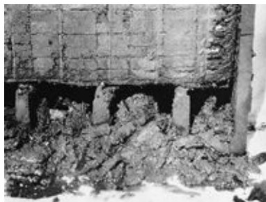
FIGURE 1-8. A severe case of shedding. The positive plate grids in
