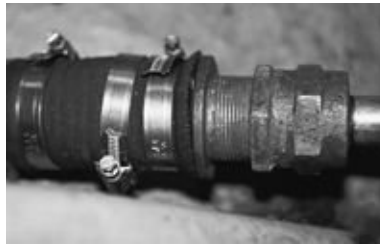
FIGURE 10-24B. A flexible stuffing box. Note the use of double hose clamps, with all 300 stainless steel construction—a quality installation.
