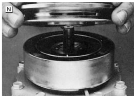
FIGURE 11-39N. Clutch installation: (1) Install the field coil. Reverse the procedure outlined in step 7, “Remove field winding.” Coil flange protrusion must match the hole in the front housing to prevent coil movement and correctly locate the lead wire. (2) Replace
