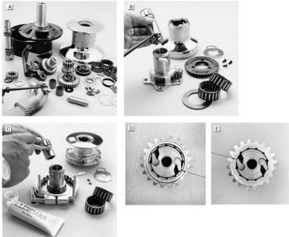
FIGURES 16-15A TO 16-15E. A large three-speed winch disassembled (16-15A). You'd better keep all the parts organized and the right way up! Oil the pawls (16-15B). Lightly grease the spindles and bearings (16-15C). Where there is a choice, make sure that ratchet gears are the right way up. Those shown in 16-15D are wrong—the pawls are not seated properly; those shown in 16-15E are correct—the pawls are fully seated. ( Lewmar )
