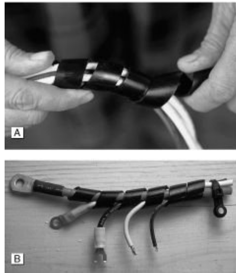
FIGURES 4-68A AND 4-68B. Plastic spiral wrap lends itself to being put on and taken off multiple times, and will expand or contract to accommodate changing wire bundle sizes.
