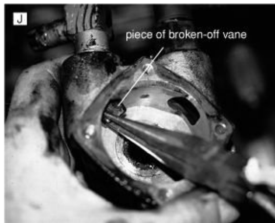
FIGURE 9-37J. Tracking down the missing vanes from the impeller shown in Figure 9-37B . The first one was found in the pump discharge elbow; the second in the tubing; and the third . . .
