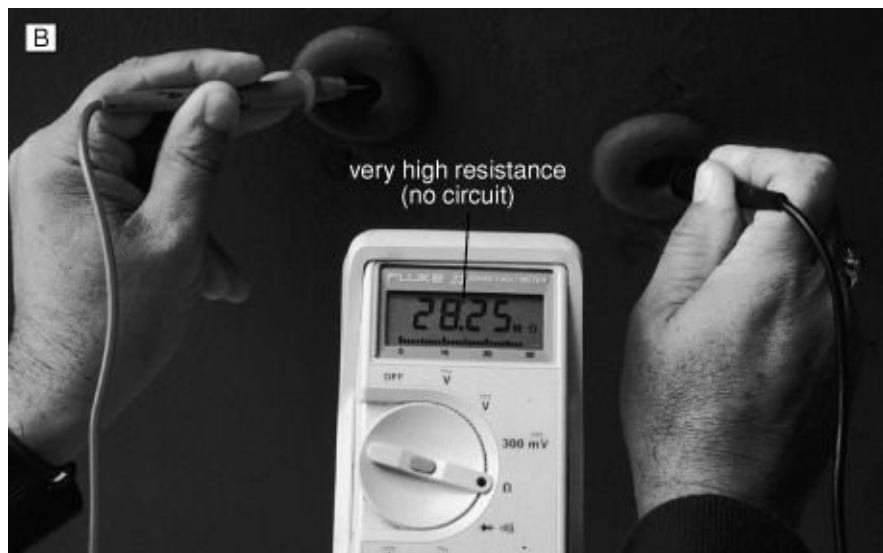
FIGURE 5-20B. Very high resistance (28.25 megaohms)
