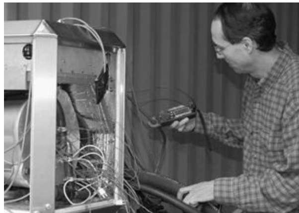
FIGURE 2-19. Kevin Alston of Glacier Bay testing a prototype Ossa Powerlite permanent-magnet DC generator.
