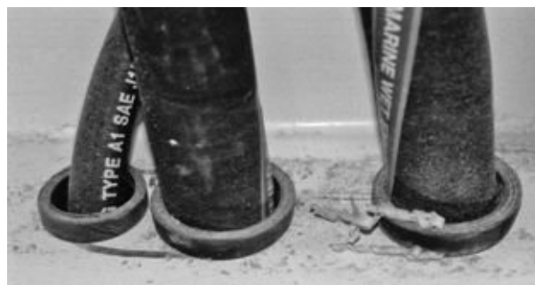
FIGURE 12-26. First-class hoses and chafe protection on our old Pacific Seacraft 40.
