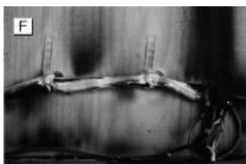
FIGURES 4-75A TO 4-75F. The effect of a dead short. This sequence of photos was taken over a couple of seconds demonstrating the catastrophic speed with which short circuits can cause major fires and render a boat uninhabitable. The cables had high-quality fire-retardant insulation, which nevertheless burned freely as long as the heat source (the short circuit) was maintained, but ceased burning
