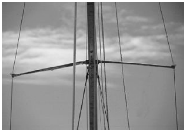
FIGURE 17-44A. A common sight. The angle made by the shrouds with these spreaders is not equal on the top and bottom sides of the spreaders (the spreader tips are too low). Under load, the spreader tips will want to slide down the shrouds, potentially bringing the mast down.
