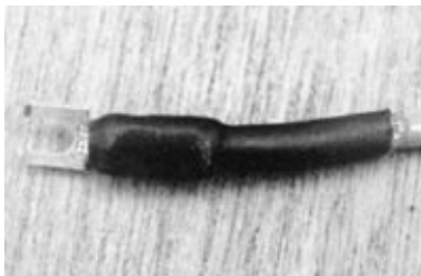
FIGURE 4-63C. The completed terminal. Note the glue squeezed out of the heat-shrink tubing. The heat-shrink sleeve will not only provide waterproofing, but also a fair measure of strain relief at the hard spot where the cable exits the terminal.
