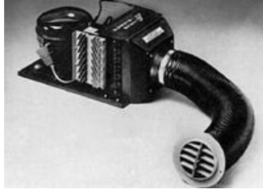
FIGURE 11-16. Constant-cycling DC refrigeration. Note the substantial air duct to the air-cooled condenser. If this becomes obstructed, or there is not an equally sized duct to disperse the hot air from the other side of the condenser, performance will suffer drastically. ( Adler Barbour )
