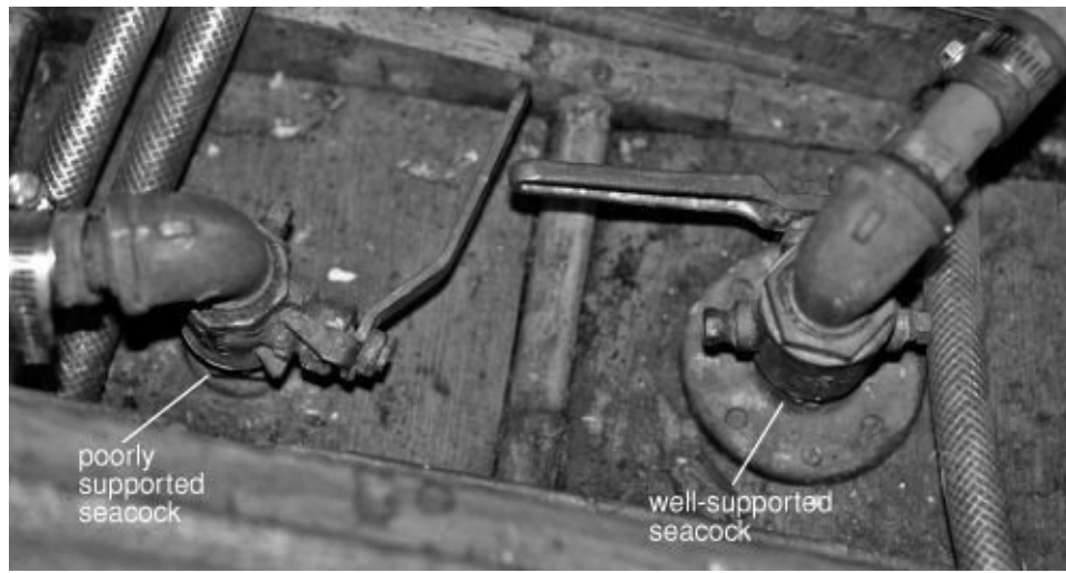
FIGURE 12-43. Proper seacocks—the position of the handle immediately shows whether they are open or closed. Note the wide load-bearing flange on one but not the other. Given that this is a relatively lightweight wooden hull, the seacock without a flange may put undue stress on the hull if ever struck hard.
