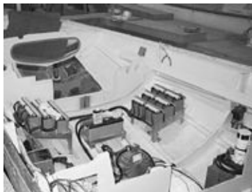
FIGURE 2-21. Solomon Technologies installation in a Hinckley DS42. There are six batteries on either side (which will be under the cockpit seats) powering the electric motor in the center. The two batteries in the center power the sail-handling hydraulic system (just visible at lower right) and have nothing to do with the electric propulsion. ( Courtesy Hinckley )
