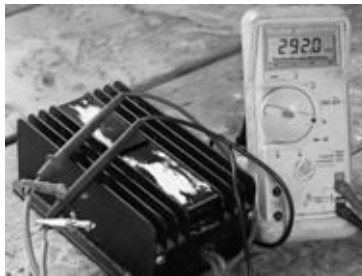
FIGURE 4-28C. Testing a galvanic isolator with a capacitor (meter used in its ohms mode). The capacitor is first discharged (by shorting the leads). The meter will build up to a high reading
