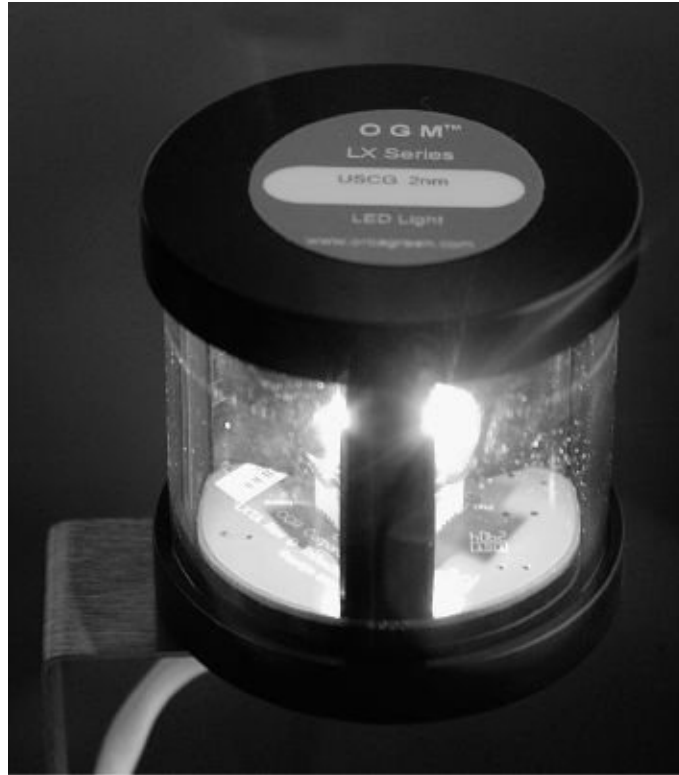
FIGURE 7-41. The OGM light shown in Figure 7-39B also includes white LEDs so that when it's used as a masthead tricolor light, it can do double duty as an anchor light.
