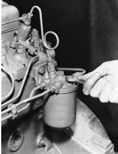
FIGURE 9-28A. Bleeding a secondary fuel filter. ( Perkins Engines Ltd. )
