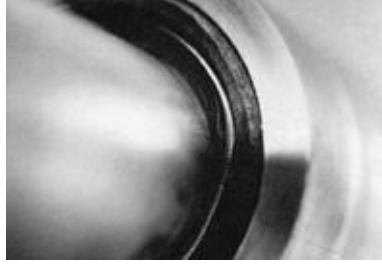
FIGURE 10-31. A rolled-over lip seal resulting from improper installation (the end of the shaft was not properly chamfered).
