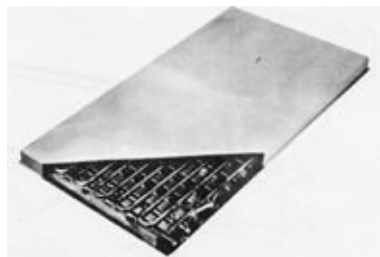
FIGURE 11-14B. A Dole Refrigerating Company holding plate. It also has a relatively closely spaced coil but in a single loop (as opposed to multiple loops in parallel). ( Dole Refrigerating Company )
