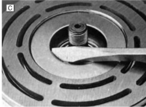
FIGURE 11-39C. For HD-series compressors, remove bearing dust cover as shown.
