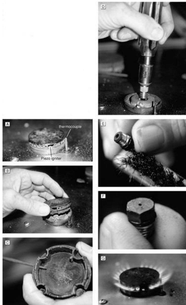
FIGURES 15-12A TO 15-12G. A burner with steadily deteriorating performance (a 3-year-old boat; 15-12A). Something has also recently boiled over on the stove top! To clean it, lift off the burner cap (15-12B). Rod out the air holes in the cap with an ice pick (15-12C). Unscrew the burner nipple/gas orifice (15-12D). Clean the orifice by poking a strand of a brass-bristle brush through it (a straightened
