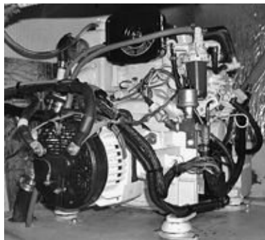
FIGURE 2-8A. A Balmar DC generator using an air-cooled, high-output alternator.
