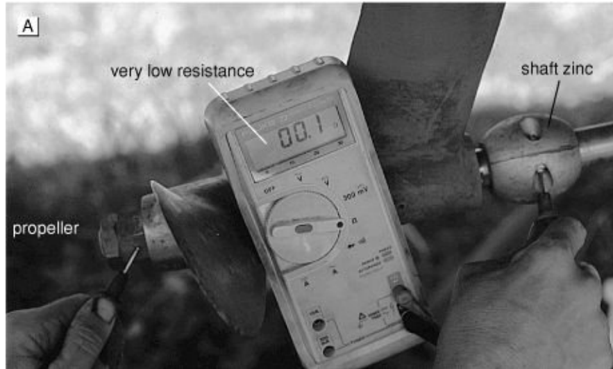
FIGURE 5-20A. The resistance between a bronze propeller and the shaft zinc protecting it and its stainless steel propeller shaft is 0.1 ohm, indicating a good connection.
