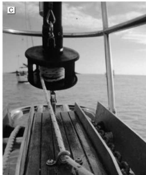
FIGURES 17-59B AND 17-59C. A block, or pad eye, set up to ensure the reefing line enters the reefing drum at the correct angle. ( Jim Sollers )
