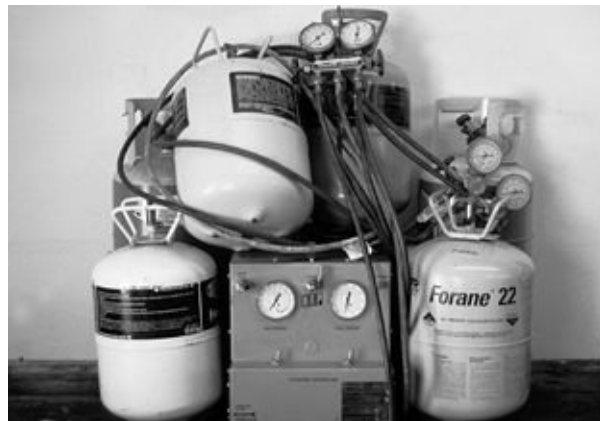
FIGURE 11-3. A collection of different refrigerants used in marine systems over the past decade, plus an EPA-certified evacuation and recovery pump.
