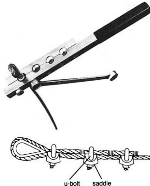
FIGURE 17-26. Although rigging eyes spliced in wire rope around thimbles are seldom seen these days, eyes retained by cable clamps or Nicopress (Talurit) sleeves are a common sight. They are just as secure as a splice, and far easier to make. Be sure to use the proper size thimble and the proper tool for crimping the sleeve, such as the portable Nicopress tool shown top right. If using cable clamps, be sure the saddle rests on the standing part of the wire rope (bottom right). (Norseman)
