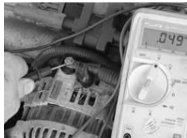
FIGURE 3-35B. Testing for AC ripple voltage from the alternator's positive terminal to negative (the alternator's case). It is very low (0.049 VAC), which is good.
