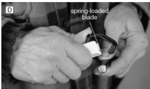
FIGURE 4-55C. Another excellent tool for stripping smaller-sized cables.
