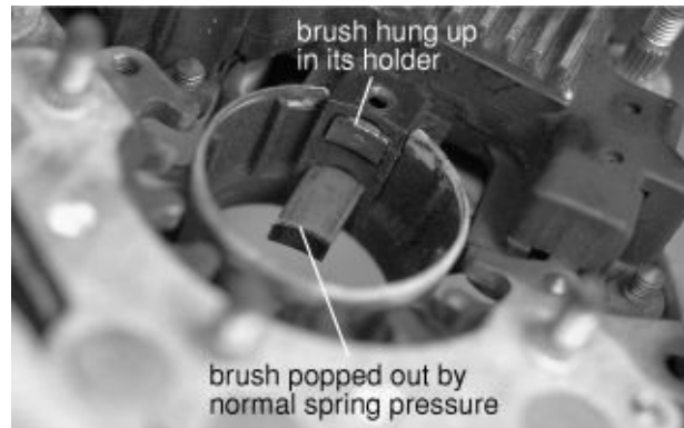
FIGURE 3-27A. A failed brush spring has caused this brush to hang up . . .
