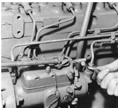
FIGURE 9-28B. Bleeding the fuel inlet pipe to a distributor-type fuel injection pump. ( Perkins Engines Ltd. )
