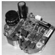
FIGURE 6-36. A maximum power point tracking (MPPT) voltage regulator, plus rectification circuits and electronic braking, in an AirX wind generator—these devices are getting pretty sophisticated! ( Southwest Windpower )
