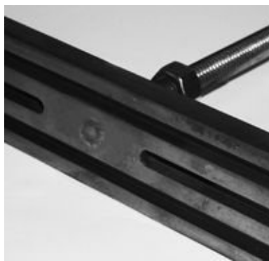
FIGURE 5-28 (left). A lightning ground plate with machined slots to maximize the edge length. There is some disagreement as to whether this has any practicable effect when the edges are relatively close together. ( Courtesy Chestnut Hill Industries )
