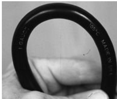
FIGURE 4-49B. Cheap cable; the only information on the insulation is “1 gauge 105°C,” which does not comply with ABYC standards.
