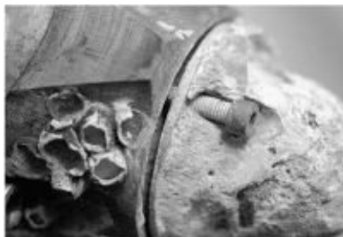
FIGURE 10-42. This zinc is past its replacement date! Note that galvanic interaction between the stainless steel fasteners and the zinc has caused the zinc to become loose. This will interfere with the
