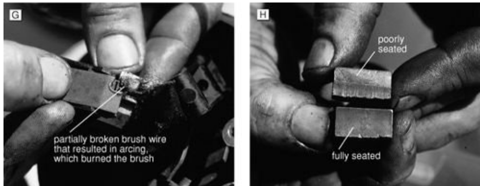
FIGURE 7-27H. A comparison of a properly seating brush with one that was never bedded in.
