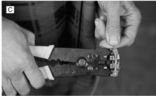
FIGURE 4-55C. Another excellent tool for stripping smaller-sized cables.
