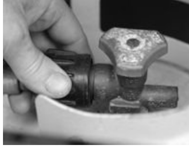
FIGURE 15-2. A U.S.-style cylinder with a quick-connect coupling. Note the OPD label below the valve handle.
