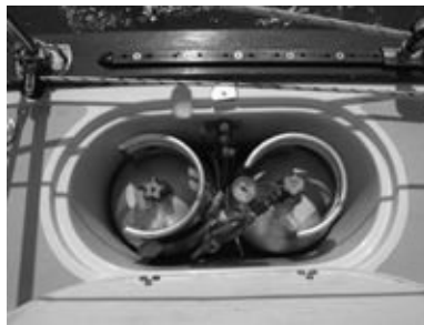
FIGURE 15-4B. An ABYC-compliant propane locker in the side
