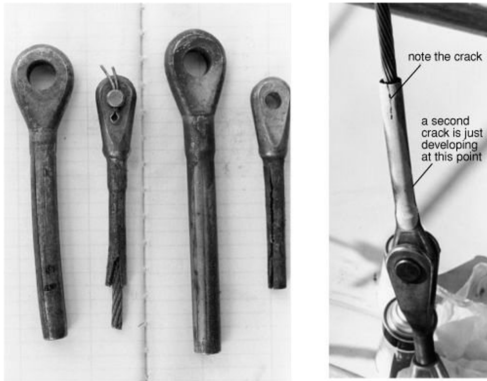
FIGURE 17-38. Stress points on hardware.
