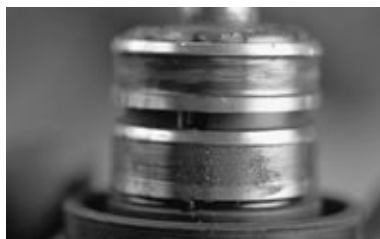
FIGURE 3-27B. . . .burning the slip ring (and also the brush, which was almost completely burned away).
