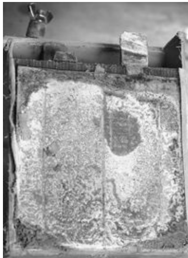
FIGURE 1-5. A dried-out gel-cell battery. This battery froze when in a discharged state, splitting the battery case and causing the electrolyte to dry out over time. (Unlike a wet-cell battery that would
