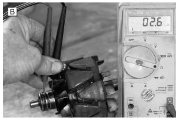
FIGURES 3-39A AND 3-39B. Rotor testing, P-type alternator, external regulator. BAT is the output terminal (leading to the battery positive terminal); FLD is the field terminal.
