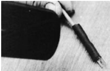
FIGURE 4-63B. Heating the heat shrink with a heat gun.
