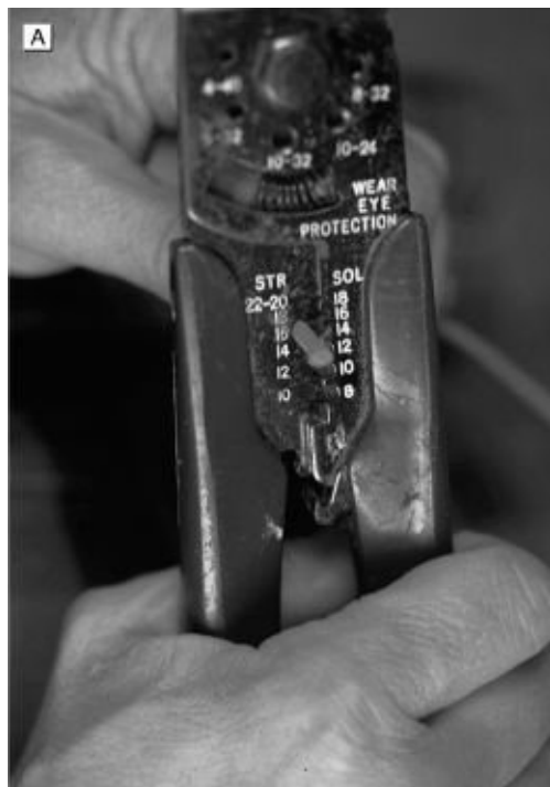
FIGURE 4-55A. A cheap wire stripping and crimping tool. Note the stripping section is labeled “STR” (for stranded cables) on one side and “SOL” (for solid cored cables) on the other side. The STR side
