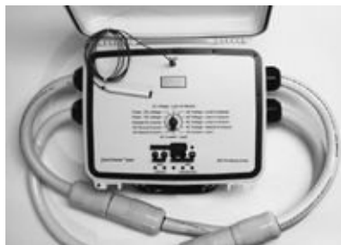
FIGURE 4-44B. A sophisticated, powerful (and expensive) test device for shore-power cords and connections. ( ESC Products Corp. )
