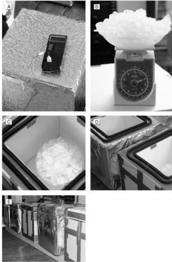
FIGURES 11-11A TO 11-11E. A 1-cubic-foot Barrier Ultra-R icebox undergoing tests (11-11A). Weighing the ice for the test (11-11B). The ice suspended over a bowl (to catch the melt water; 11-11C). Note the double seals on the icebox lids. The icebox in the background (11-11D) has an outer layer of Heat Shield. Five iceboxes in a test (11-11E). Note the thermocouple wires coming out of each box to measure the internal temperature and calculate the temperature differential with the ambient temperature.
