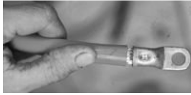
FIGURE 4-59C. The finished crimp. A little too much insulation was cut off this cable; it would be better if the insulation butted up to the terminal.
