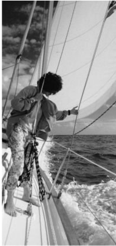
FIGURE 17-47. Testing the leeward shrouds for tension when close hauled in 10 knots of wind.
