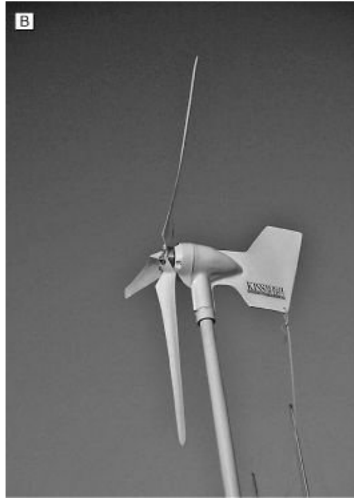
FIGURE 6-31B. A Kiss wind generator, which has no slip rings. The cord hanging from the tail limits the number of times it can turn in order to protect the output cables from damage.
