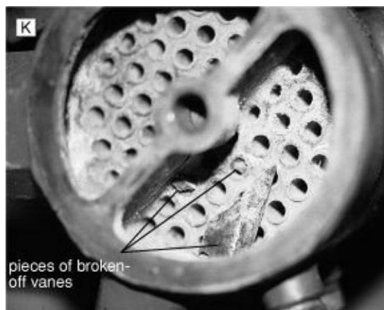
FIGURE 9-37J. Tracking down the missing vanes from the impeller shown in Figure 9-37B . The first one was found in the pump discharge elbow; the second in the tubing; and the third . . .
