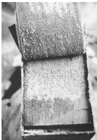
FIGURE 1-14. A dried-out gel-cell as a result of overcharging. The liquid has been driven out of the electrolyte, leaving a dry powder.
