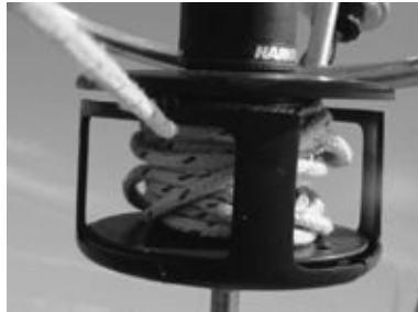
FIGURE 17-59A. A riding turn on a drum as a result of the reefing line not being fed onto the drum at 90 degrees.
