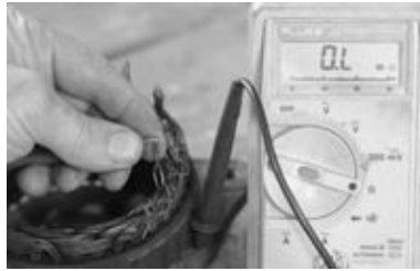
FIGURE 3-41A. Testing from a stator winding to ground (the alternator case). There should be an open circuit (O.L.—very high resistance).
