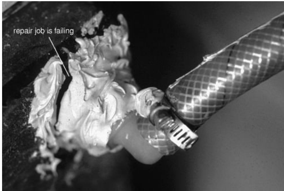
FIGURE 12-7. This vent fitting on a holding tank broke when stepped on. A repair was attempted with polyurethane sealant, but nothing sticks too well to polyethylene.
