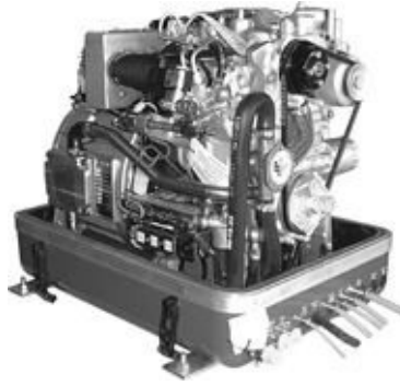
FIGURE 7-6. A Fischer Panda generator with a water-cooled stator. These generators have a high output relative to their weight.
