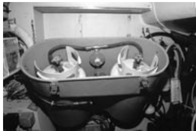
FIGURE 15-4D. An ABYC-compliant, commercially made propane locker for retrofitting boats with propane.
