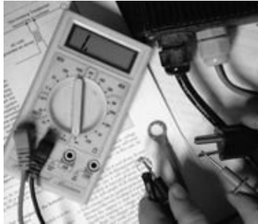
FIGURE 6-13B. Testing from an AC inlet prong on the AC cord of a battery charger to the DC output cable. There should be no continuity (displayed on this meter as “1.”).
