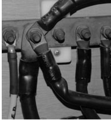
FIGURE 6-28B. A heavy copper bus bar serving as the boat’s main negative bus bar. There is severe discoloration on the connections as a result of corrosion in the marine atmosphere. Tin plating would greatly enhance the corrosion resistance.
