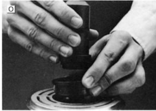
FIGURE 11-39O. Using the rotor installer set, place the ring part of the set into the bearing cavity. Make certain the outer edge rests firmly on the outer race of the rotor bearing. Now place the tool set driver into the ring as shown.
