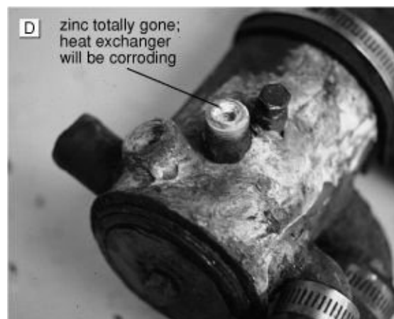
FIGURE 9-14C. This zinc should have been replaced long ago. The heat exchanger is likely corroding.
