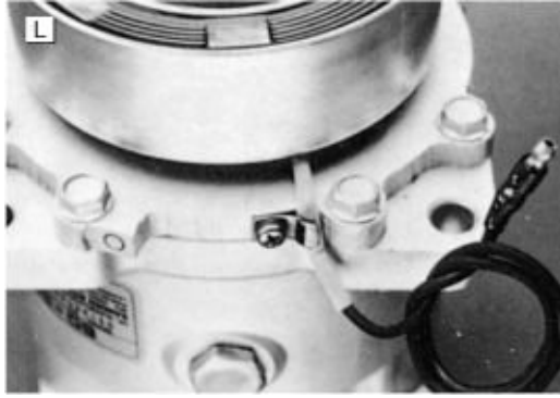
FIGURE 11-39L. 7. Remove field winding; if necessary, loosen winding lead wire from its clip on top of compressor front housing.
