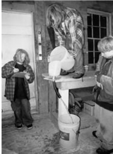
FIGURE 13-11. Kitchen sink flow rate experiments through a 1-foot length of 1-inch ID hose. It confirmed the flow rate numbers in the U.S. Navy Salvor's Handbook .
