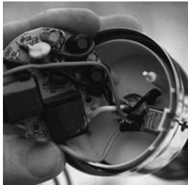
FIGURE 7-36. There are no user-serviceable parts here. If a CCF light fails, the entire unit must be replaced.
