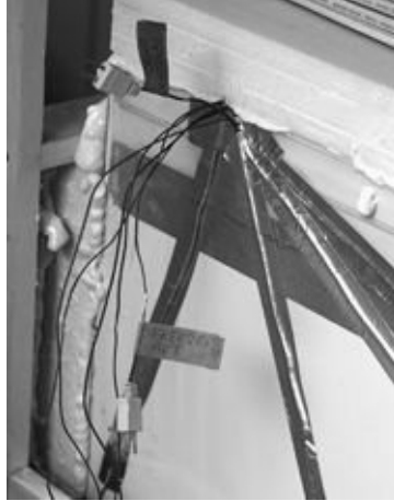
FIGURE 11-10. Thermocouples taped to all the Barrier Ultra-R vacuum insulation panels from which my new icebox is built.
