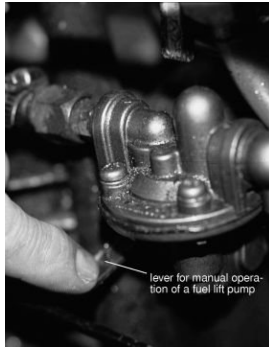
FIGURE 9-26B. Manual operation of a lift pump on a Yanmar.
