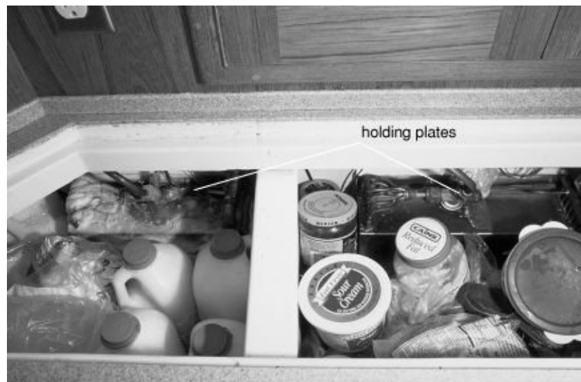
FIGURE 11-22B. Holding plates in the icebox on our old Pacific Seacraft 40, driven by a Glacier Bay ½ hp DC unit.
