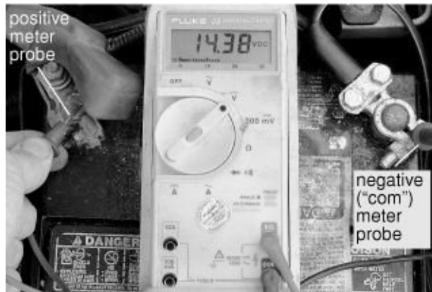
FIGURE 3-30B. Checking the absorption voltage at the battery.
