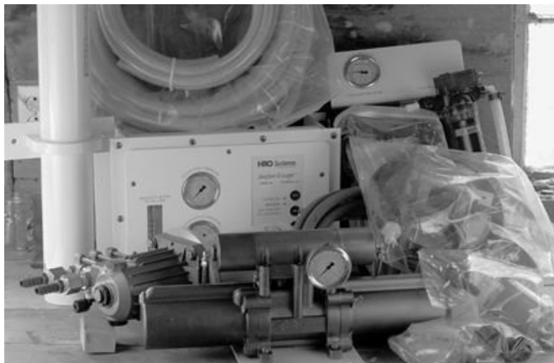
FIGURE 13-37A. All the components for a modular watermaker. This gives some sense of the large number of pieces, hose connections, etc.
