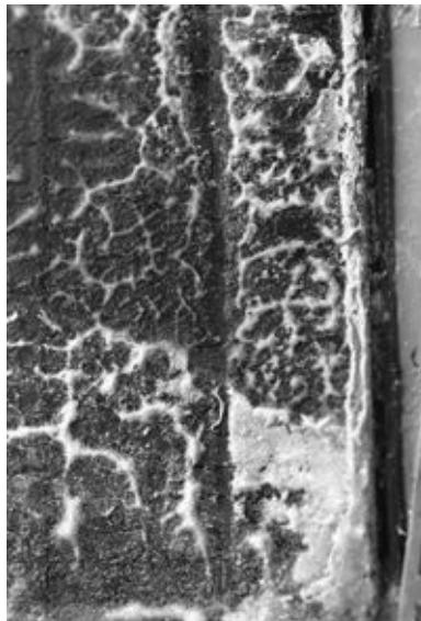
FIGURE 1-4. Paste-like consistency of the electrolyte in a gel-cell battery.
