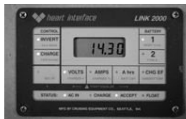
FIGURE 3-14. Sophisticated metering, including amp-hours, built for Heart Interface by Cruising Equipment Company (now part of the Xantrex group). ( Heart Interface )
