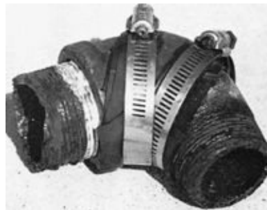
FIGURE 9-15B. The same corroded exhaust elbow patched with rubber inner tube and hose clamps. This repair held for 200 hours of engine-running time.
