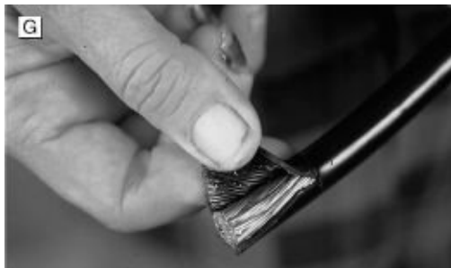
FIGURES 4-55D TO 4-55G. An insulation stripper for large cables. A small spring-loaded blade cuts through the insulation. It is run around in a circle and then dragged sideways to cut a slit in the insulation, which is then peeled off.
