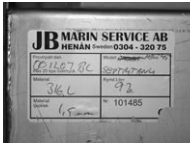
FIGURE 12-5A. The label on a holding tank being installed in our new boat. Note that the tank is 316L stainless steel. Nevertheless, I am not happy with the use of metal tanks . . .
