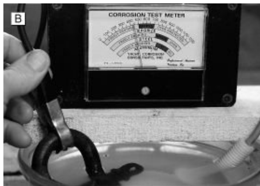
FIGURE 5-2A. The natural voltage of a galvanized anchor swivel with respect to a reference metal (in this case a silver/silver chloride half cell) is here around 960 millivolts (the voltage of the zinc coating).
