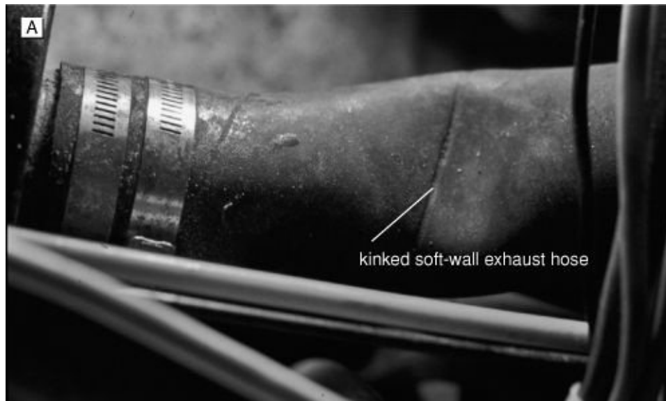
FIGURE 12-15A. Sagging soft-wall exhaust hose. When it gets hot, it sags some more, significantly interfering with the exhaust flow and engine performance at higher engine loads.
