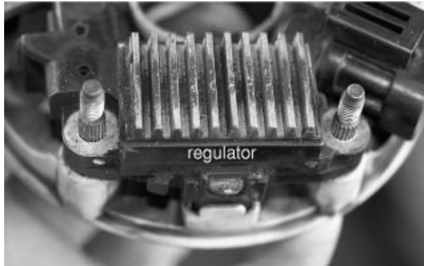
FIGURE 3-42B. Another regulator inside an alternator. This one has no accessible wiring.
