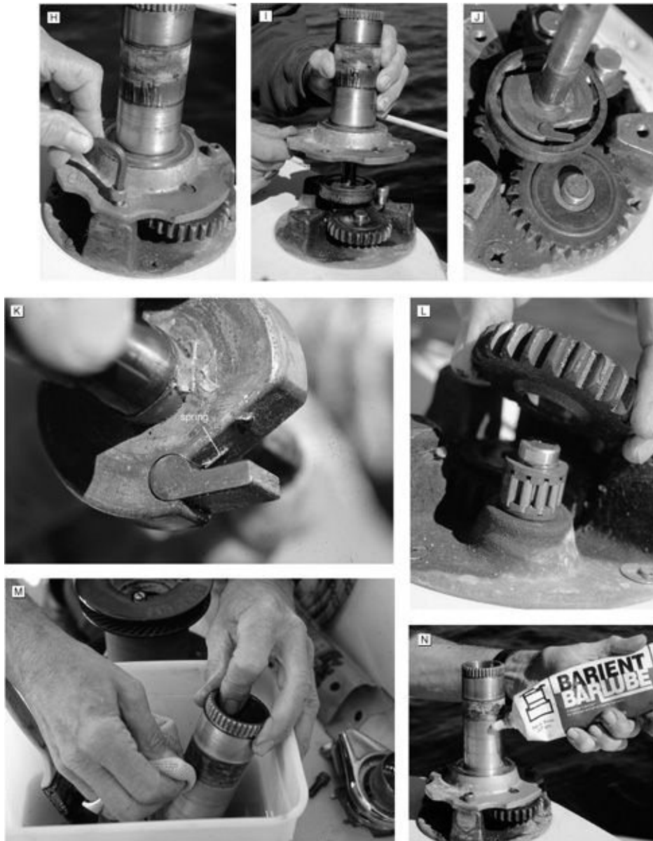
FIGURES 16-13A TO 16-13N. Disassembling a Barient winch. Use a deck-plate key to unscrew the top of the winch (16-13A). Remove the top plate (16-13B), allowing the stripper arm to be lifted off (16-13C). Next comes the drum (16-13D). The drum bearings are a little grungy (16-13E). The center stem above the surface on which they seat is somewhat corroded, but this will not affect winch performance (nothing seats on this part of the surface). Lift off the drum bearings (16-13F). Use a winch handle locked in place to pull out the spindle (16-13G; be careful as the last of it comes out—there may be spring-
