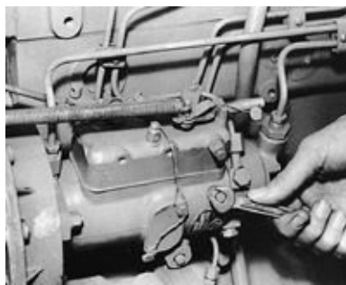
FIGURE 9-28D. Bleeding the upper nipple on a distributor-type fuel injection pump. ( Perkins Engines Ltd. )
