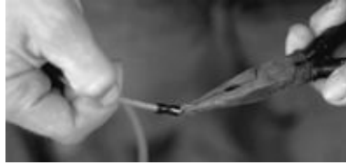
FIGURE 4-58. Tugging on a terminal to make sure it is well attached.
