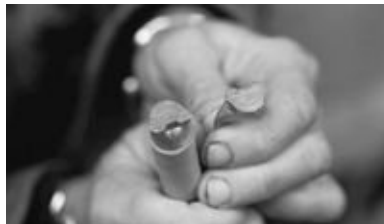
FIGURE 4-60. The crimp in Figure 4-59C cut in half, demonstrating the high degree of compaction of the cable strands (it looks like solid copper).
