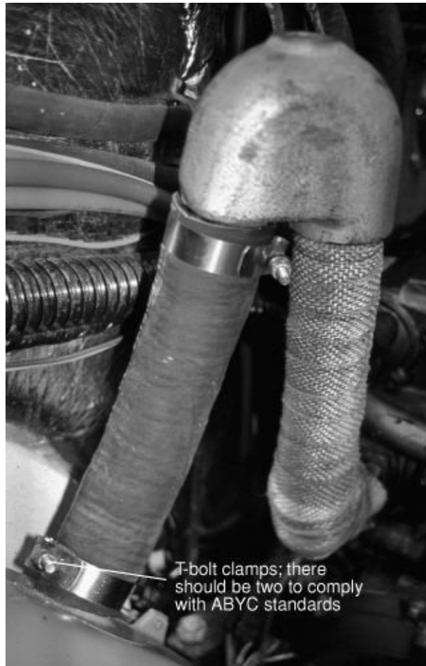
FIGURE 12-16. T-bolt clamps on an exhaust. However, the single clamps do not comply with ABYC standards.
