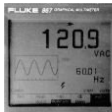
FIGURE 6-18E. The sine-wave output from an inverter also maintains a very stable voltage and frequency.
