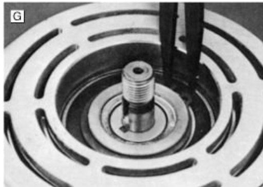
FIGURE 11-39G. 5. Remove the external front housing snap ring by using snap ring pliers (spread type).
