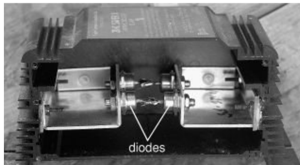
FIGURE 4-26A. A galvanic isolator—showing the two sets of counterposed diodes—without a capacitor.
