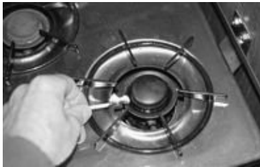
FIGURE 15-14. A little alcohol in the cup around the burner is used to preheat the burner, vaporizing the fuel in its internal channels.
