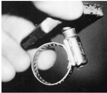
FIGURE 5-6B. An “all-stainless” hose clamp with a screw of an inferior (magnetic) corrosion-prone grade of stainless.
