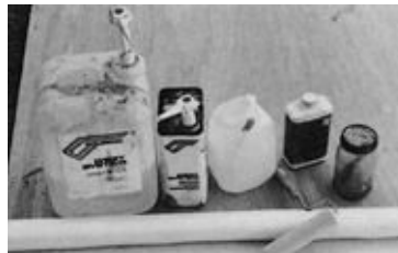
FIGURE 3-6C. The ingredients: plywood, fiberglass cloth (which will give a smoother, more finished appearance than fiberglass mat or woven roving), epoxy resin and hardener, a roller and brush, acetone for cleaning tools, and a mason jar for saving used acetone.
