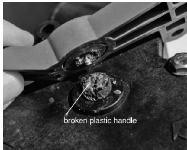
FIGURE 12-45. A broken plastic Y-valve handle.
