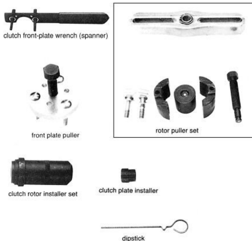
FIGURE 11-38. Special tools used in servicing Sanden compressors. ( Sanden International )
