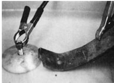
FIGURE 5-10A. A test rig to simulate stray-current corrosion. Here 5 amps of DC current are being passed from the stainless steel flat bar to the zinc anode via the electrolyte (salt water).
