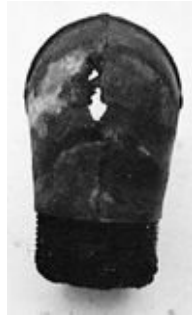
FIGURE 9-15A. A corroded galvanized exhaust elbow. The hot gases and water from the engine exhaust have eaten right through it.
