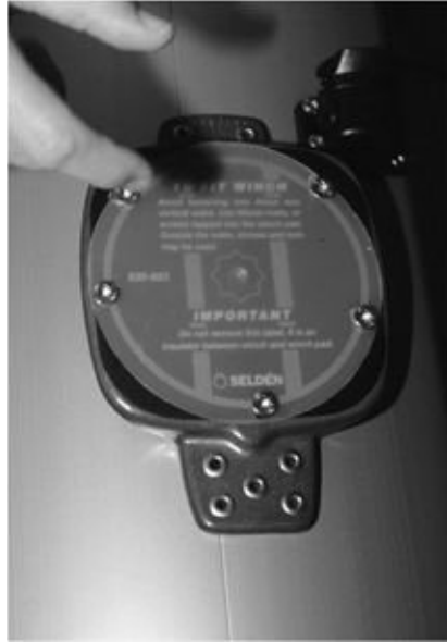
FIGURE 17-13B. A winch pad on a Selden mast. It comes with a galvanic insulator already installed.
