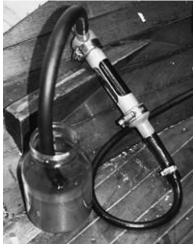
FIGURE 9-7A. Pumping a fuel sample from the base of a tank.
