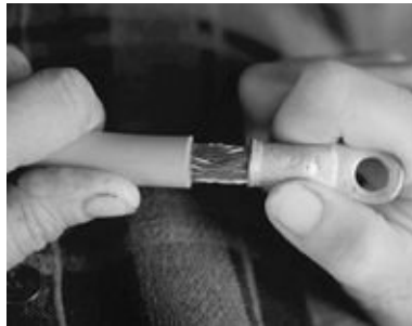
FIGURE 4-53. Larger sizes of Type 3 cable (multistranded) are often a tight fit in their terminals and sometimes hard to get in without clipping a few strands.
