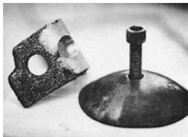
FIGURE 5-10B. After less than 3 hours, the stainless steel is severely corroded, whereas the zinc is unharmed.
