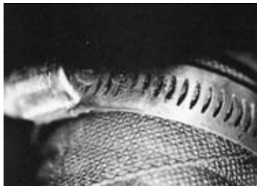
FIGURE 5-6C. A perfectly good-looking “all-stainless” hose clamp, which, when the screw was backed off a turn or two, revealed considerable corrosion inside the screw housing, caused by using an inferior grade of stainless steel for the screw.
