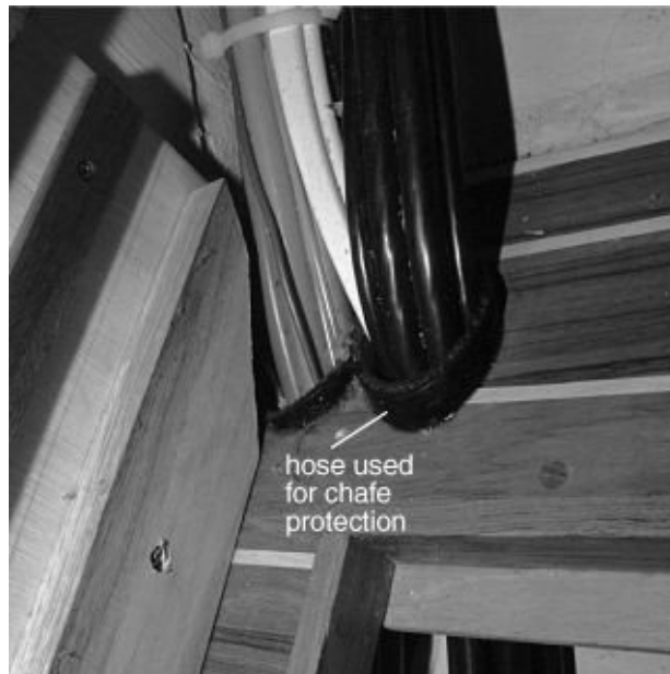
FIGURE 4-67B. Excellent chafe protection (using hoses) on our old Pacific Seacraft 40.
