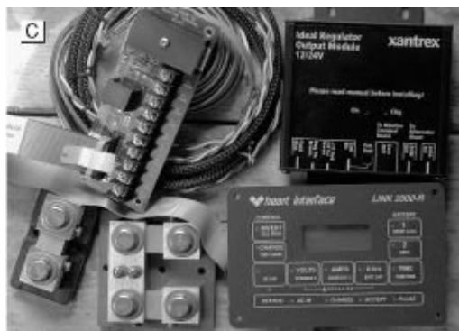
FIGURE 1-40C. A complete DC monitoring system, including two shunts (one for battery amps, the other for alternator amps), a
