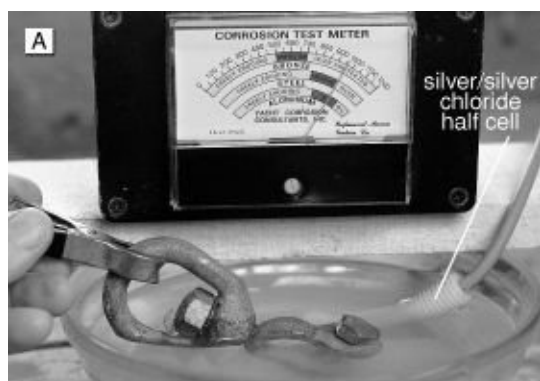
FIGURE 5-2A. The natural voltage of a galvanized anchor swivel with respect to a reference metal (in this case a silver/silver chloride half cell) is here around 960 millivolts (the voltage of the zinc coating).
