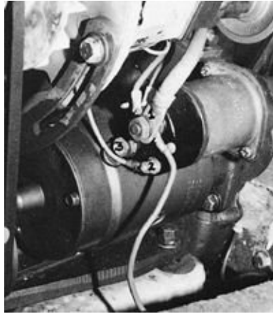
FIGURE 7-24A. A typical preengaged starter motor and solenoid. Jumping across 1 and 2 bypasses the ignition switch; 1 and 3 bypasses both the ignition switch and the solenoid. The starter should spin but will not engage the engine's flywheel.
