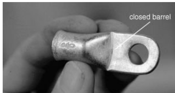
FIGURE 4-52. Note the closed barrel, which will prevent moisture wicking up into the cable.
