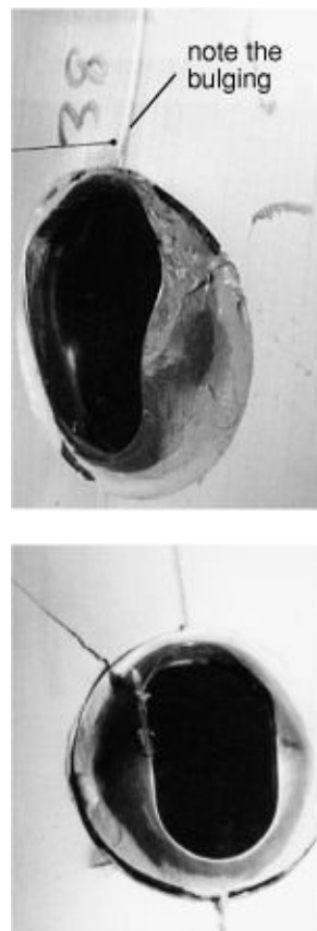
FIGURE 17-21. Check for these trouble spots around the shroud socket area of a mast wall: mast wall distorted by T-ball shroud socket (top), and mast wall cracked by shroud socket (bottom).
