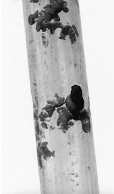
FIGURE 5-5. Crevice corrosion on a stainless steel propeller shaft caused by stagnant water with low oxygen content in the stern tube.
