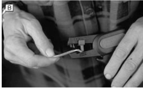
FIGURE 4-55B. A useful tool for stripping smaller cable sizes. The plastic stop can be set to ensure just the right amount of insulation is taken off.
