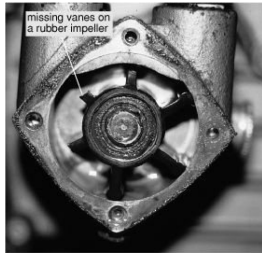
FIGURE 9-37B. A raw-water pump with its cover removed. Three out of six vanes on the impeller are missing!
