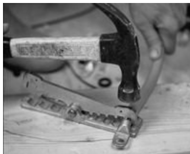
FIGURE 4-59B. A cheap but effective crimping tool for large cables.
