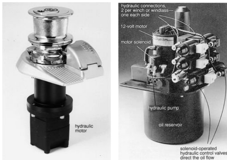
FIGURE 16-33. A hydraulic windlass (left) and an electrically powered hydraulic power pack (right). Solenoid-operated hydraulic control valves (upper right on the power pack) direct oil to the winch through the connectors (two per winch; one each side). ( Lewmar )
