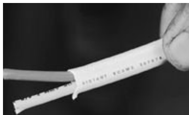
FIGURE 4-49C. Quality cable again—BC5W2—that is also oil resistant (the label is partially cut off). Although it cannot be seen in
