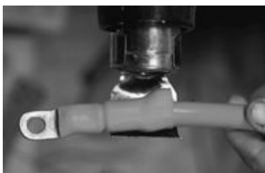
FIGURE 4-63D. Heat shrink being applied to a large cable. The
