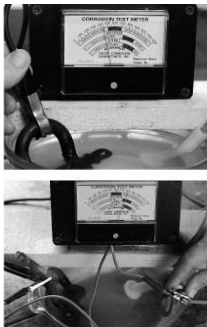
FIGURES 5-16A AND 5-16B. A steel shackle, once again, at its natural voltage of around 440 millivolts. When wired to an immersed galvanized shackle, the voltage potential jumps to that of the zinc coating on the galvanized shackle (810 mV). The zinc is now being sacrificed to protect the steel shackle.
