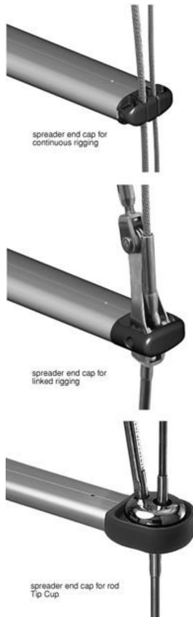
FIGURE 17-44B. Spreader tip arrangements. Top: A mechanism for locking continuous wire rigging in place. Middle: Discontinuous wire rigging using swaged terminals. Bottom: Discontinuous rod rigging with stemball fittings. ( Selden )
