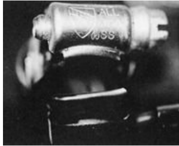
FIGURE 5-6D. A good-quality all-stainless hose clamp using a 300-grade corrosion-resistant screw.
