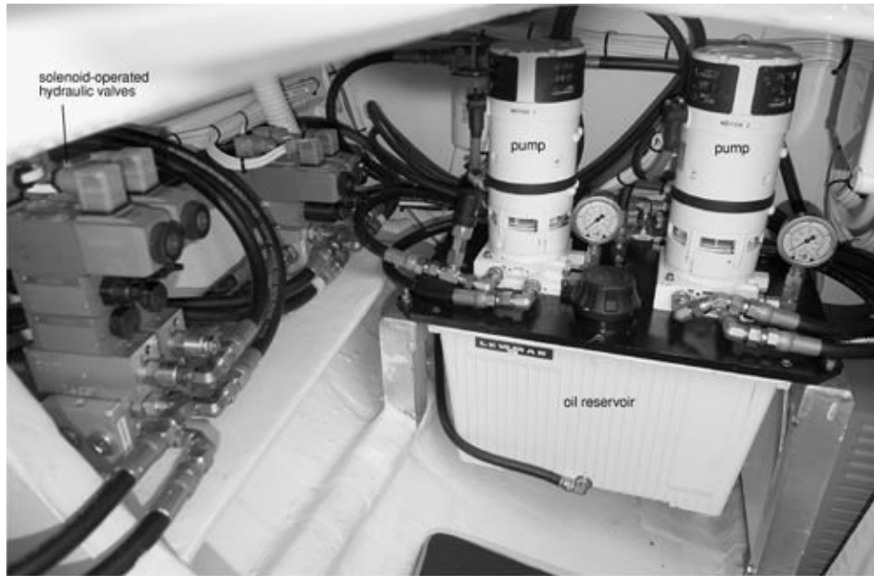
FIGURE 16-34. A Lewmar hydraulic system as installed. The solenoid valves that direct hydraulic oil to various hydraulic motors are on the left; the two pumps and the oil reservoir are on the right.
