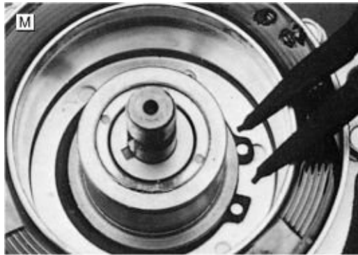
FIGURE 11-39M. Use spread-type snap ring pliers to remove snap ring and field coil.
