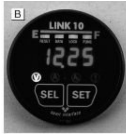
FIGURE 1-40B. A basic systems monitor, resembling the fuel gauge in a car.
