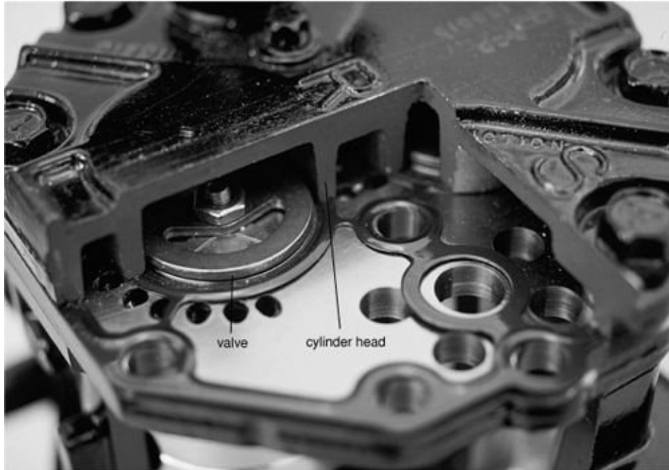
FIGURE 11-41B. The valves, which are accessed by removing the cylinder head.
