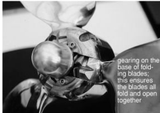
FIGURE 10-39C. The geared hub of a contemporary folding propeller.
