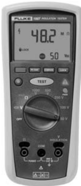
Figure 11.30 Measuring insulation resistance. (a) Simplified circuit diagram for insulation-resistance tester (megohm-meter); (b) insulation and continuity tester
