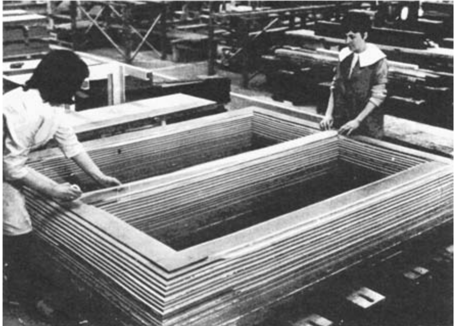
Figure 7.15 (a) Typical core cross-section for large transformer; (b) packs of laminations being laid up to form shaped core
