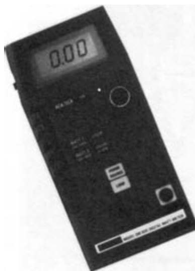
Figure 11.20 Digital wattmeter with key selection of functions and ranges
