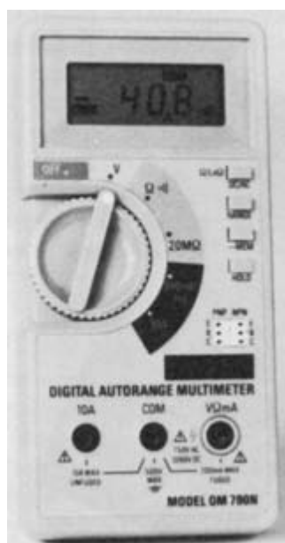
Figure 11.19 Three-digit autoranging multi-meter with memory and hold facilities
