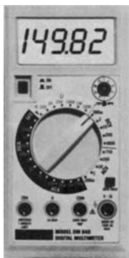
Figure 11.17 Four-and-a-half-digit electronic multi-meter with switch selection of ranges
