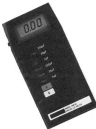
Figure 11.21 Digital L/C meter with key selection of functions and ranges
