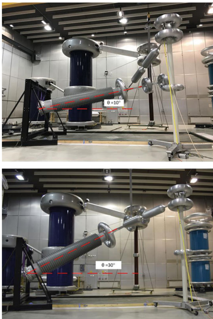
Fig. 5.27 Setup with different cross-arm segment inclined angles in the water induced corona discharge test
