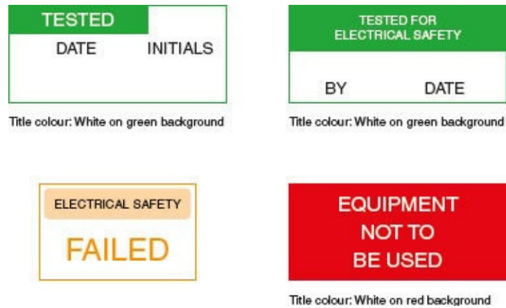
Figure 1.32 Typical PAT Test labels.
