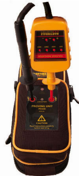
Figure 1.27 Voltage indicator being proved.
