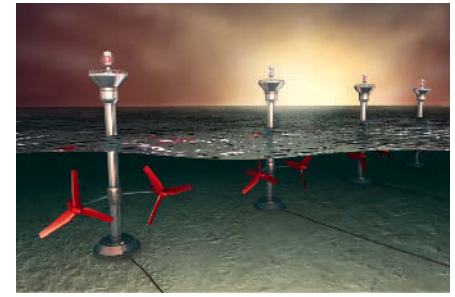
Figure 3.23 Tidal flow water turbines.
