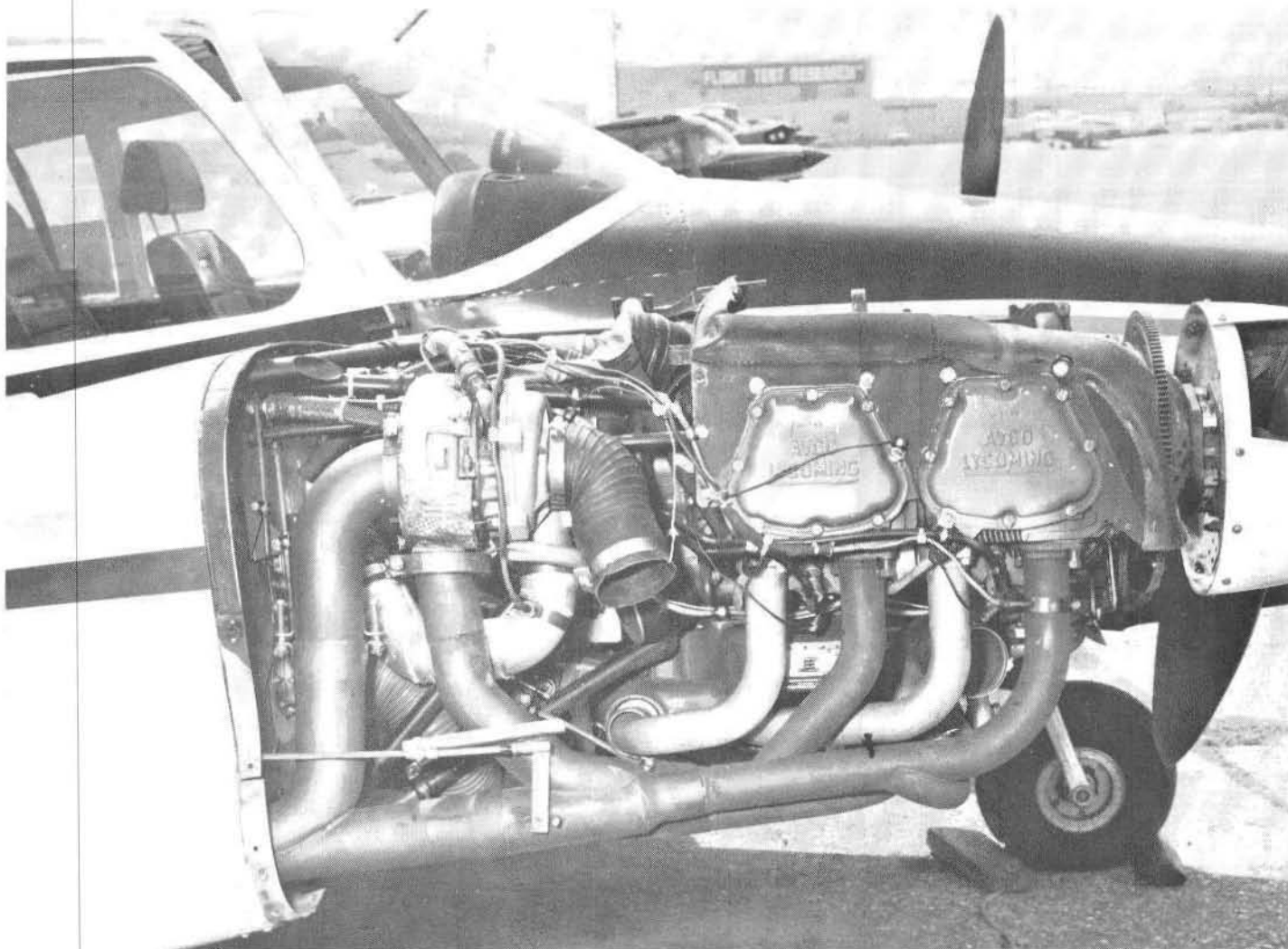
Piper Seneca is a light twin. This version has Rajay aftermarket kits on Lycoming Engines. Factory-turbocharged Continental engines on later versions are also Rajay turbocharged.
