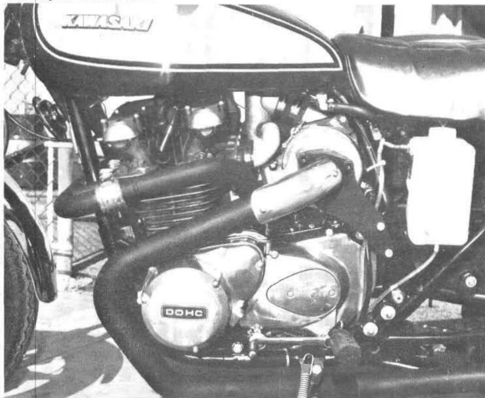
Figure 162—900 Kawasaki Turbocharger kit by Blake Engineering uses a Model 377B.25 Rajay Turbocharger. Installation is capable of over 30 pounds boost. Water injection is also used.
