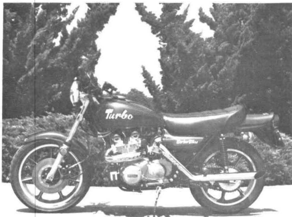
Figure 158—Turbocharged performance of 500cc Honda with American Turbo-Pak kit
