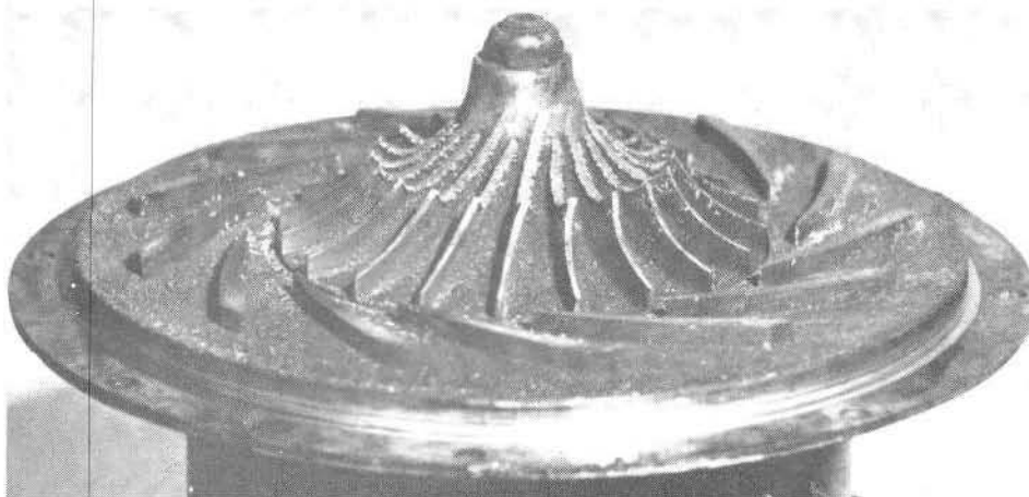
Figure 135—Compressor impeller failure caused by foreign object
