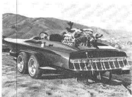
Tom Scahill installation on a 454 CID Chevrolet includes his own aftercooling equipment which he sells to other marine enthusiasts. Kits include carburetor box, intercooler, Rajay turbochargers and AiResearch waste gate.
