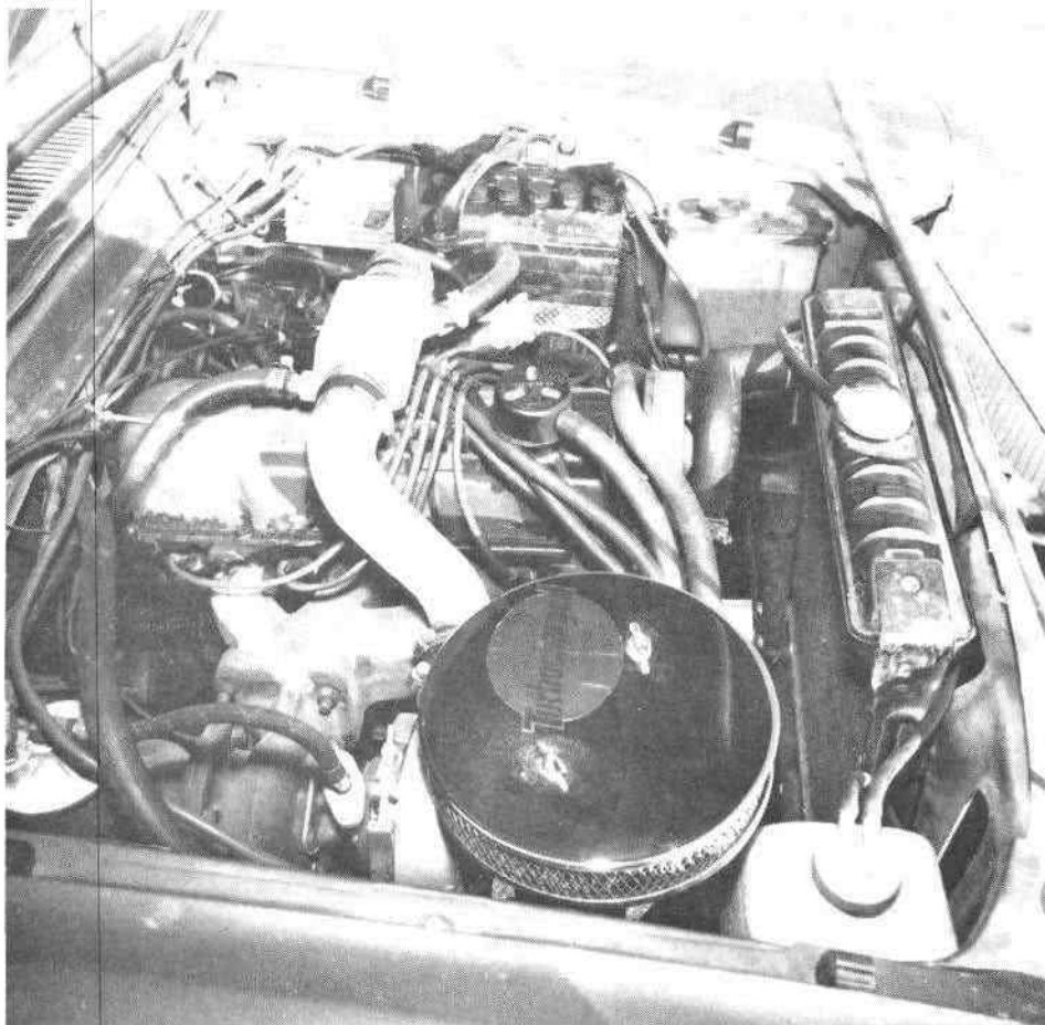
Ak Miller uses jacket water to heat long crossover pipe on 2-liter Pinto installation. Special exhaust manifold mounts turbocharger.
