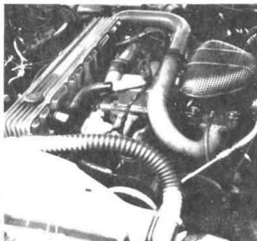
Toyota has taken their 1600 twin cam, which was originally an optional engine for the Celica (domestic market), stretched it to 1800cc's and is now offering it in three stages of tune: One with dual 44mm Solexes, one fuel injected and then the full route with a turbocharger. With the dual Solexes they claim 145 HP. Fuel injection runs it up about another ten ponies, but they won't say what they get out of the turbocharged unit. Bob Dunham photo.
