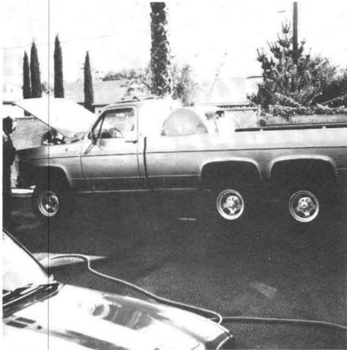
Nick Trist of Hidden Hills, California had this GMC pickup modified for off-road use. It has six-wheel drive and air suspension all around. He had Ak Miller add propane and two turbochargers to give it passenger-car performance.
