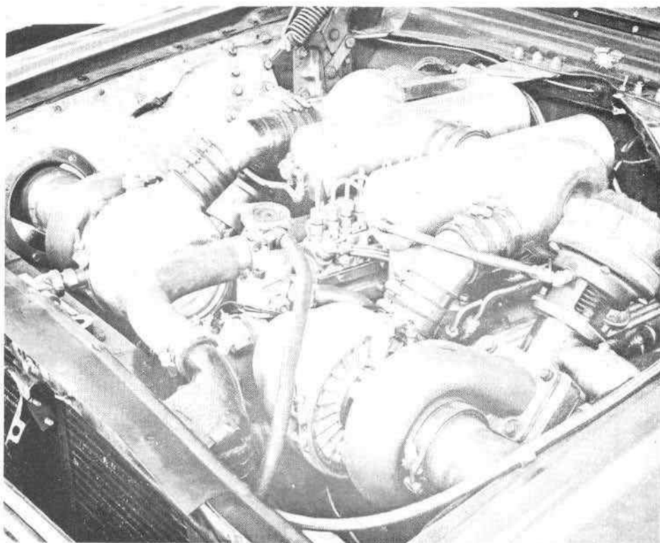
Chevy small-block V-8 installation in a Ford Ranchero used exclusively for speed runs at Bonneville Salt Flats. Cragar machinist Bill Edwards owns the car and made the installation of two AiResearch TE0659 turbos with waste gates. Note plenums, Bosch fuel injection.
