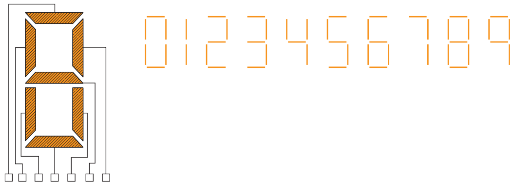
Figure 9.84 LED used in seven-segment display.
