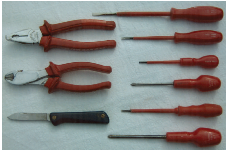
Figure 5.17 The tools used for making electrical connections.
